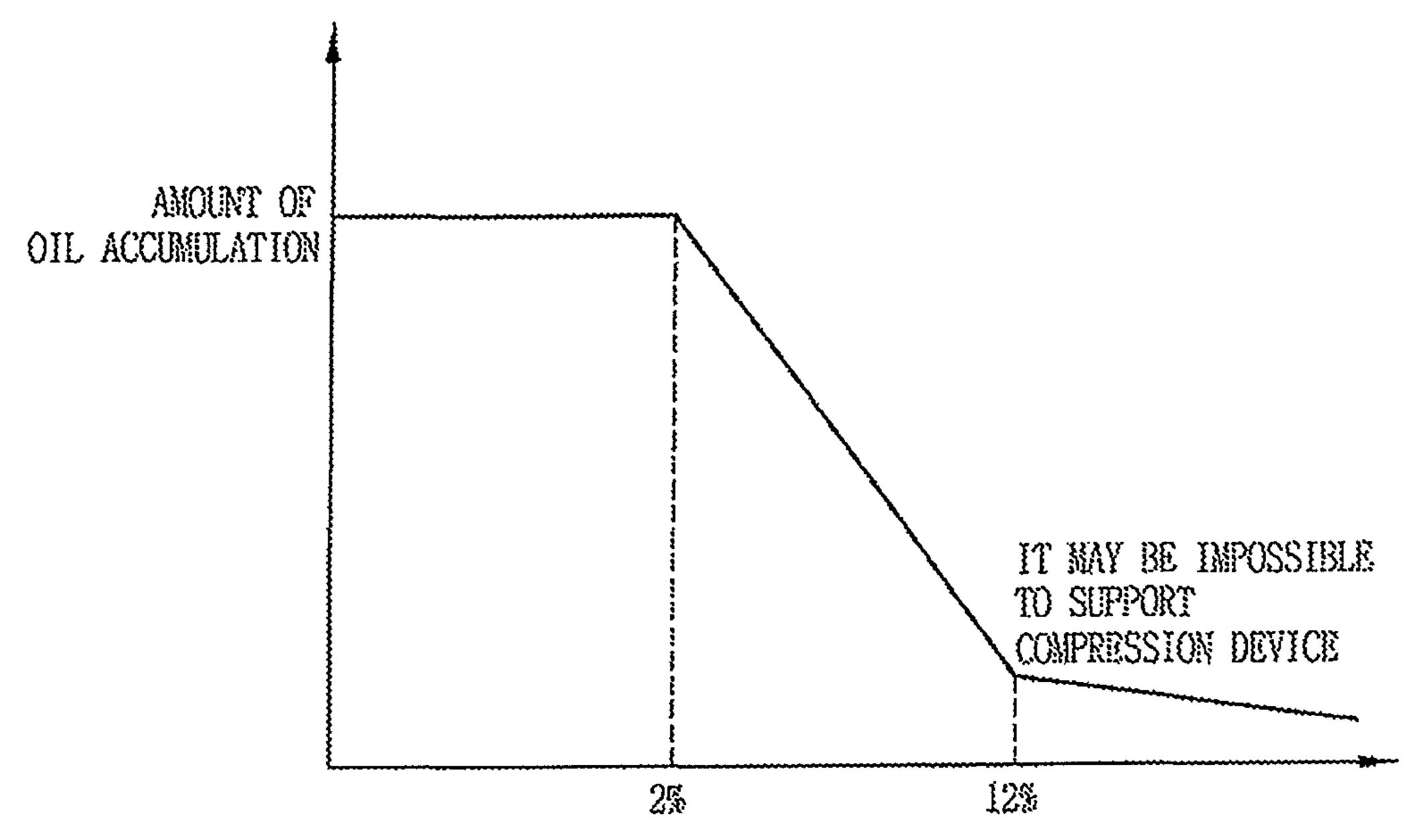
CROSS-SECTIONAL AREA RATIO OF OIL DISCHARGE PATHS (CROSS-SECTIONAL AREA OF OIL DISCHARGE PATHS/ INNER DIAMETER CROSS-SECTIONAL AREA OF CASING)
