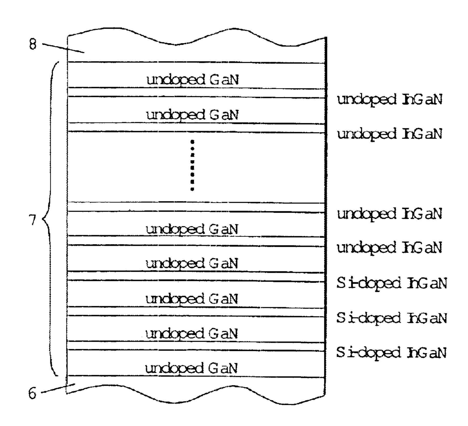
well structure with large number of layers and relatively low forward voltage, especially with an improved emitting effi-
