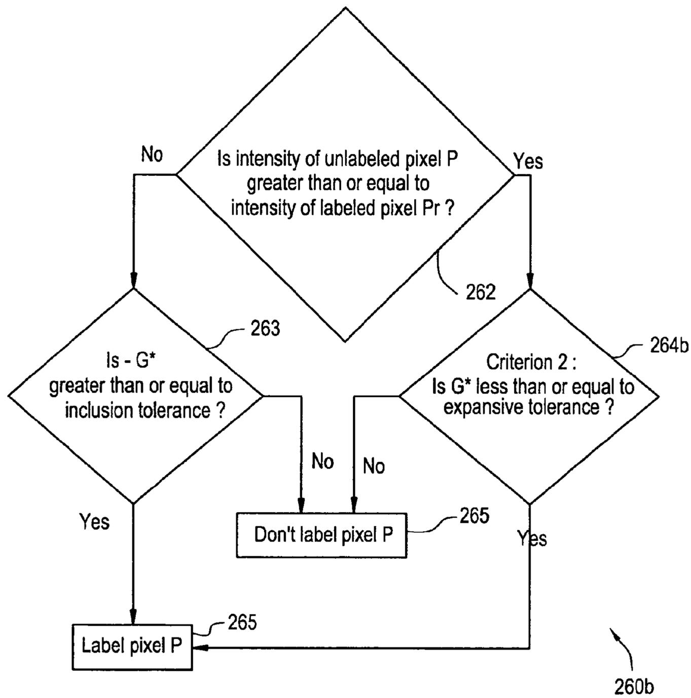
\*G = d( P0, P ) - d ( P0, Pr ) = difference in distances from local maximum P0 to unlabeled point P and labeled point Pr
