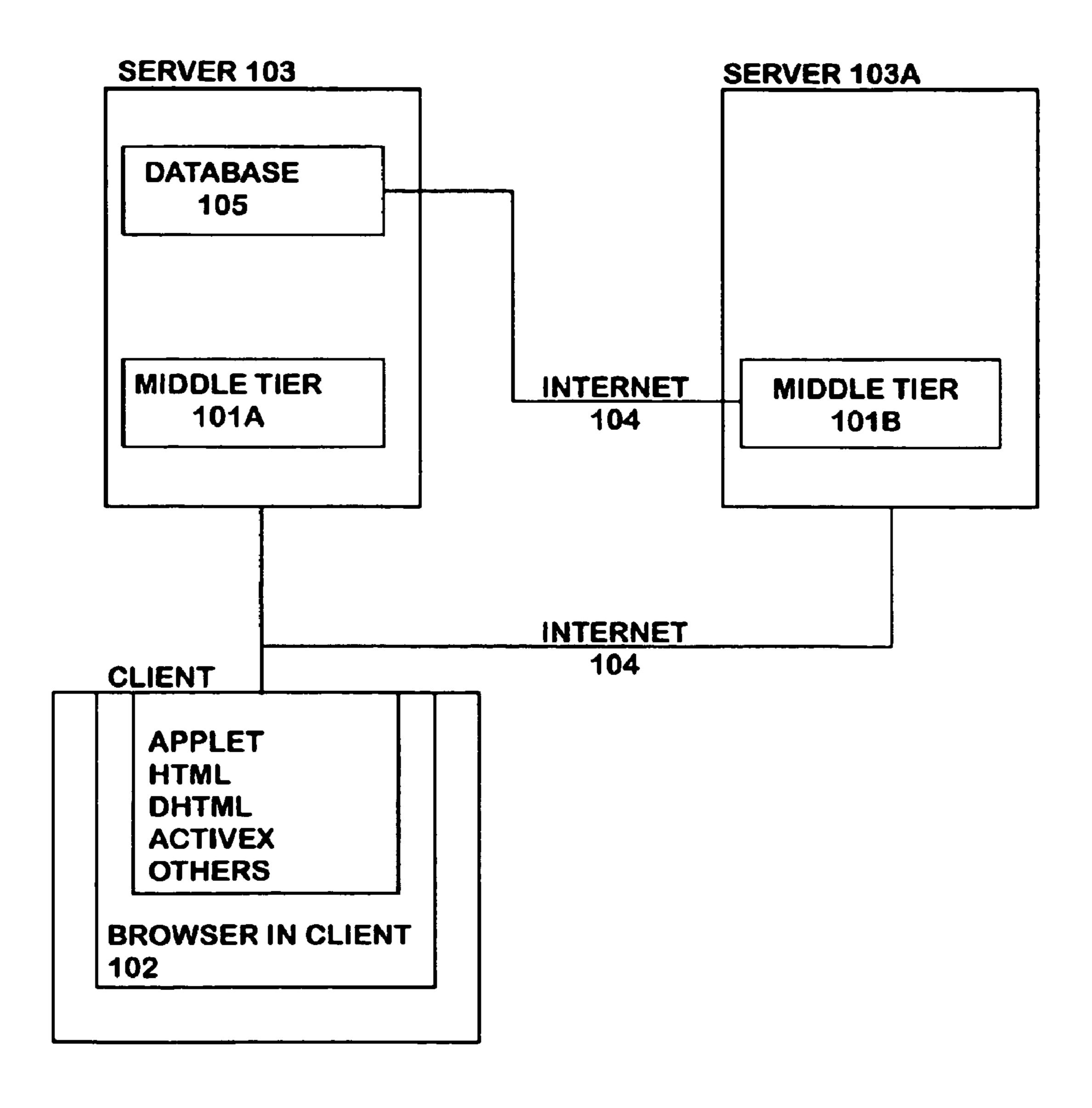
THE MIDDLE TIER CAN EITHER BE IN THE SERVER COMPUTER THAT CONTAINS THE DATABASE, OR CAN BE IN ANOTHER SERVER COMPUTER THAT COMMUNICATES OVER THE INTERNET TO THE SERVER IN THE DATABASE. THE SERVERS CAN COMMUNICATE WITH THE BROWSER USING HTML, JAVA APPLETS, DHTML, ACTIVEX OR OTHER INTELLIGENT COMPONENTS OF THE BROWSER.
