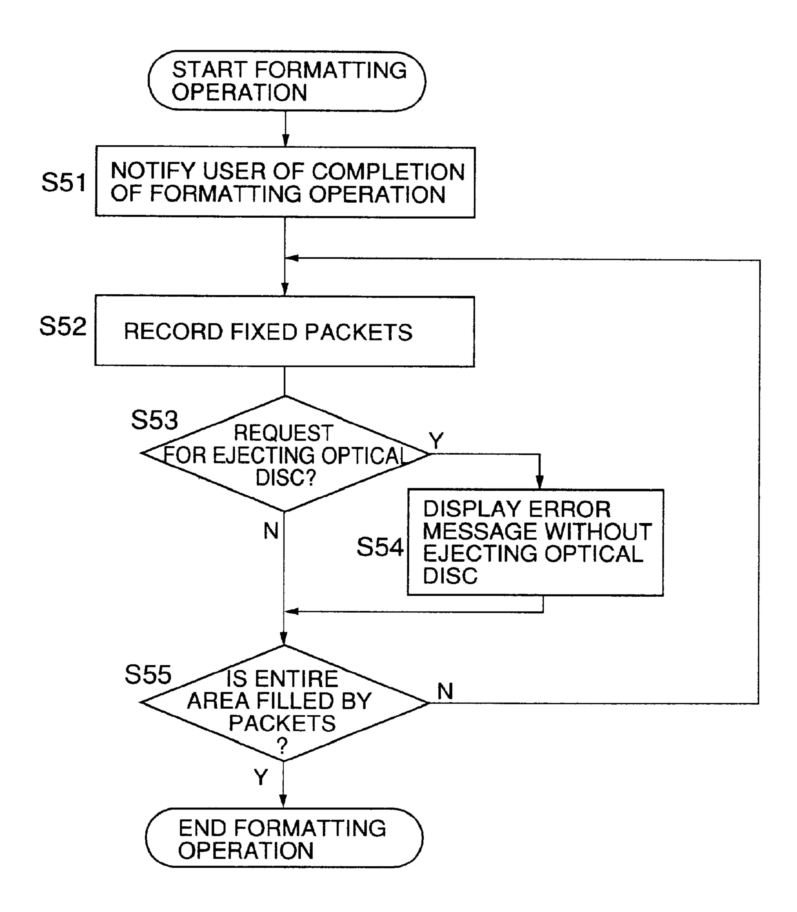
OPTICAL DISC RECORDING AND REPRODUCING APPARATUS FOR PERFORMING A FORMATTING PROCESS AS A BACKGROUND PROCESS AND A METHOD FOR FORMATTING AN OPTICAL DISC BY A BACKGROUND PROCESS
