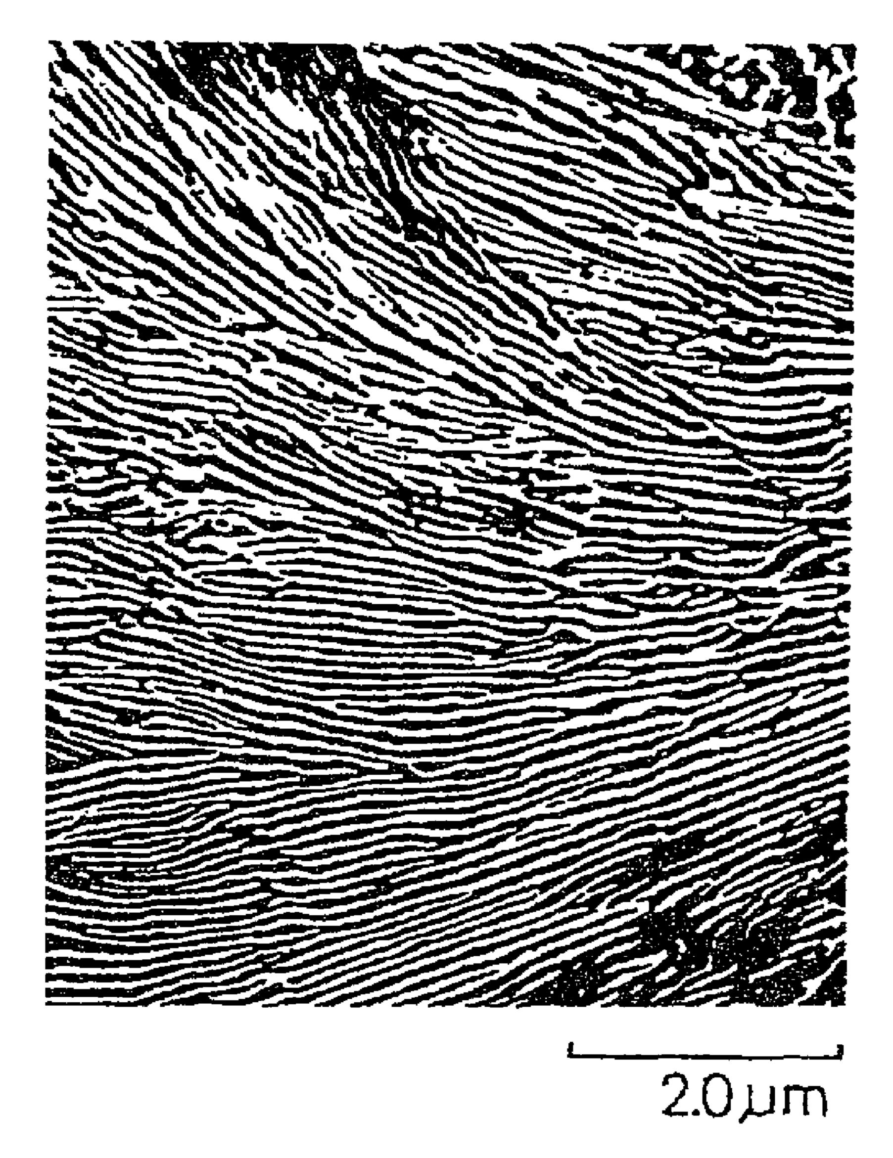
RAIL STEEL OF THIS INVENTION (No. 8)  $\lambda = 0.77 \text{ nm}$  Rc = 0.19
