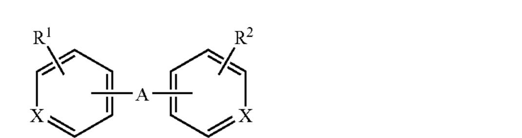
wherein, A represents *sulfide group*, *disulfide group or* bivalent aliphatic hydrocarbon residue which may be optionally interrupted by imino group, [sulfide group, or disulfide group,] X represents nitrogen atom or C(NH<sub>2</sub>), and R<sup>1</sup> and R<sup>2</sup> independently represent hydrogen or alkyl.
