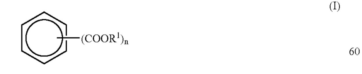
(wherein R<sup>1</sup> represents an alkyl group having 6 to 16 carbon atoms, and n represents an integer of 1 to 6) and (b) 0 to 80% by weight of another base oil with (c) 65 0.1 to 10% by weight, based on the total amount of the lubricant composition, of an antioxidant.
