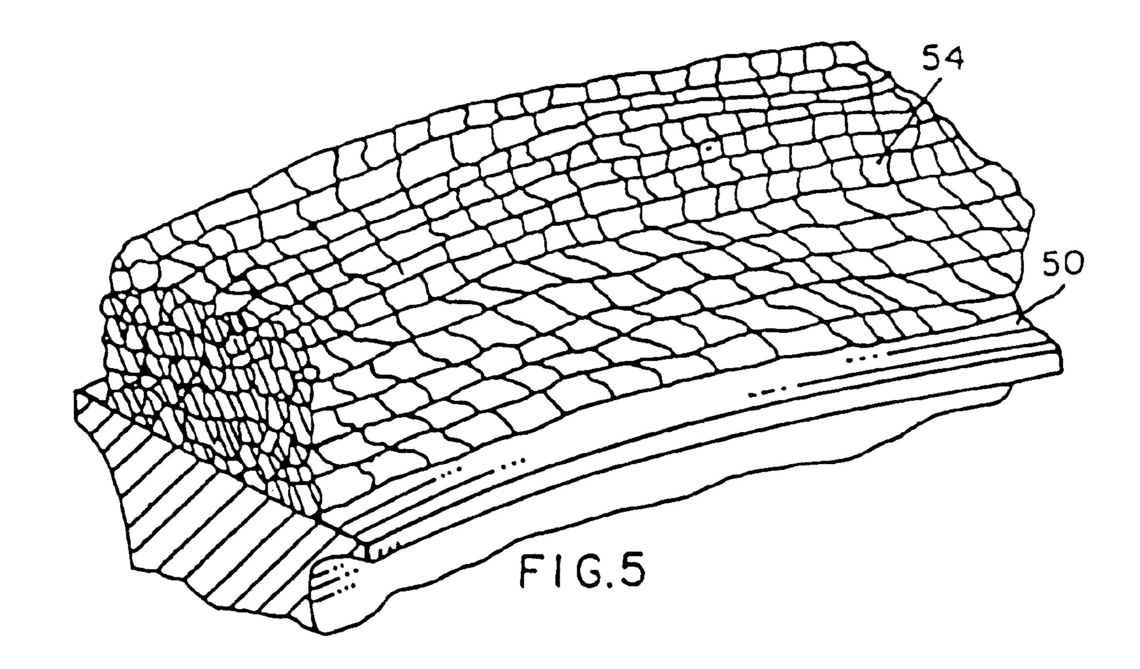
TURBINE SYSTEM HAVING MORE FAILURE RESISTANT ROTORS AND REPAIR WELDING OF LOW ALLOY FERROUS TURBINE COMPONENTS BY CONTROLLED WELD BUILD-UP
