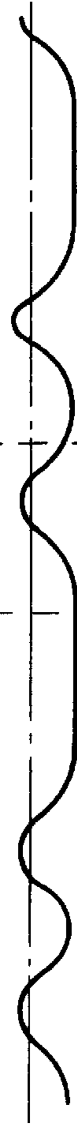
OUTPUT SIGNAL OF AIR FUEL RATIO SENSOR 9 AND COMPARISON LEVEL 2
