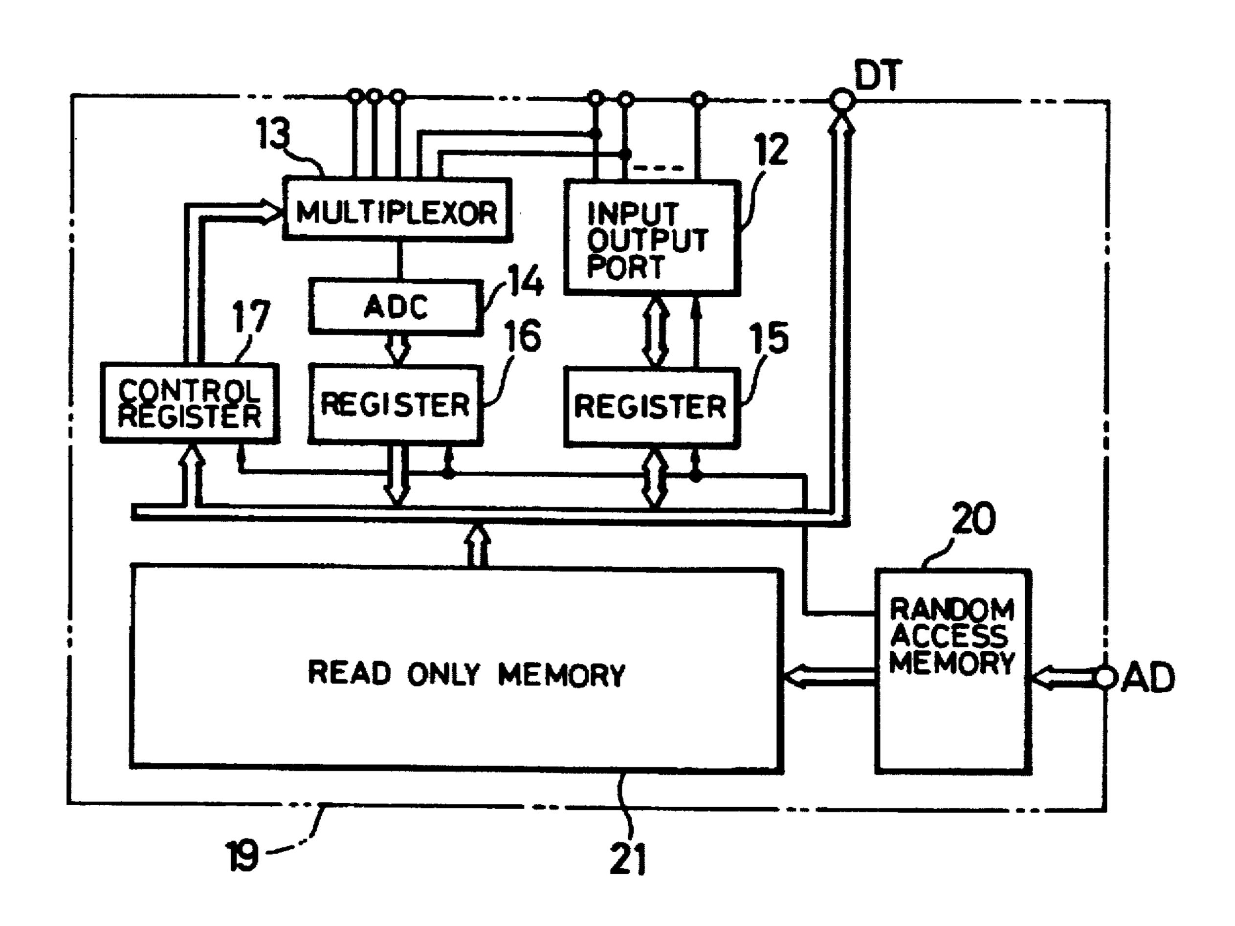
MONOLITHIC INTEGRATED CIRCUIT HAVING COMMON EXTERNAL TERMINAL FOR ANALOG AND DIGITAL SIGNALS AND DIGITAL SYSTEM USING THE SAME
