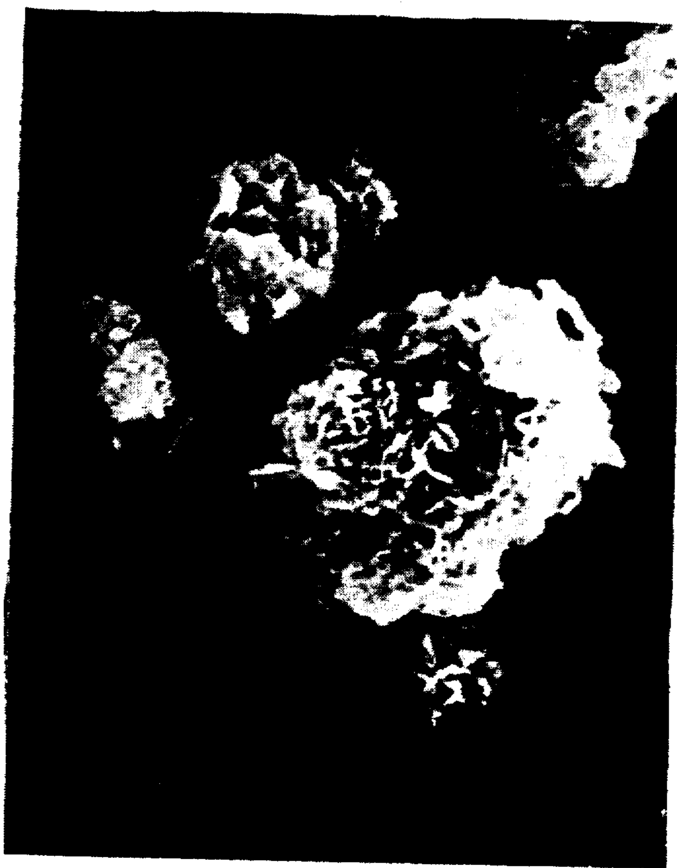
SYNTHETIC HYDROTALCITE (5000 X)
