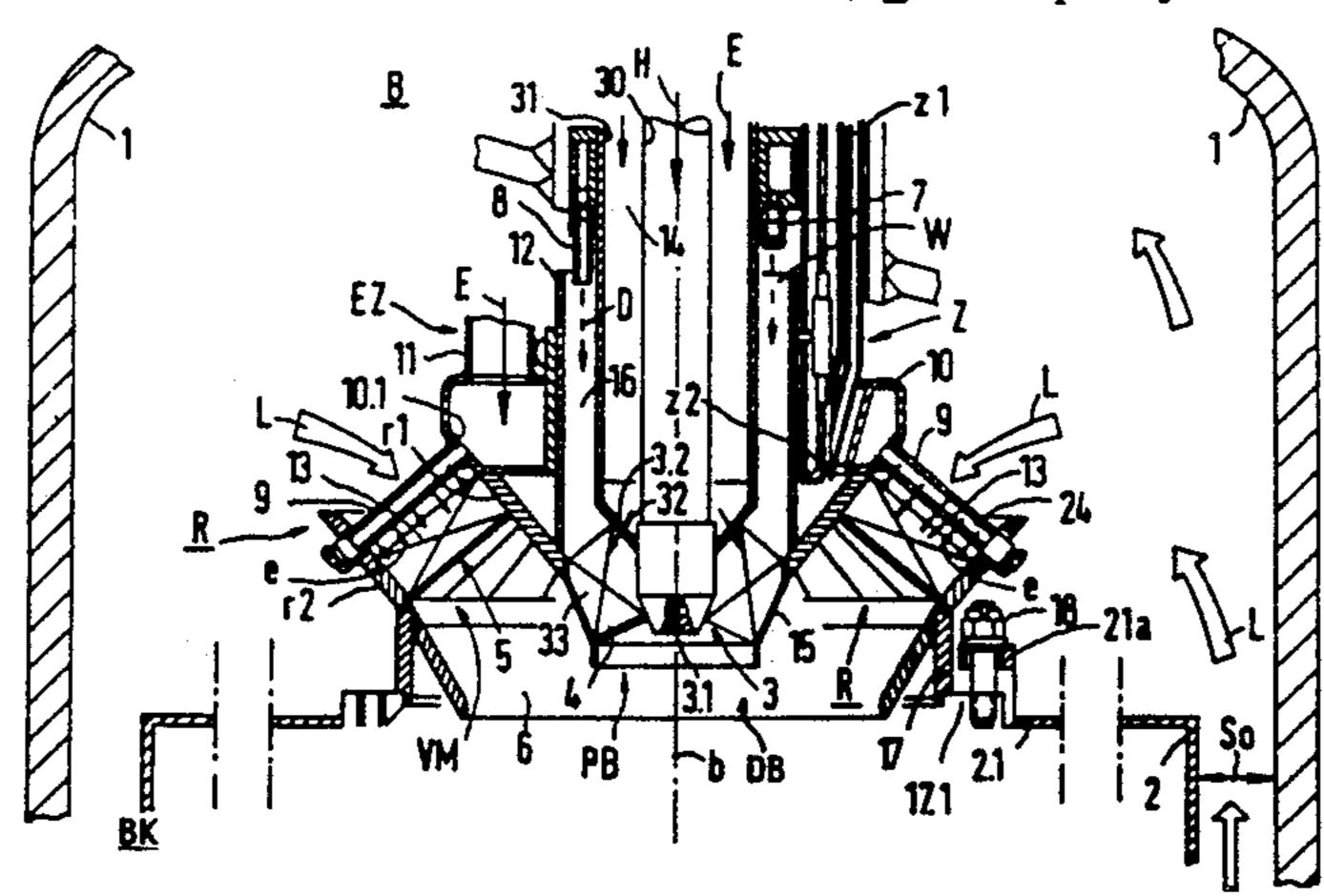
inflow cross section in a direction substantially transverse to the flow direction, the nozzle tubes each having a side with nozzle openings facing away from the air inflow side of the ring channel system, a device defining nozzle openings disposed in the ring channel system, and a [natural] gas feeding system [substantially concentrically surrounding the pilot burner and] con-
