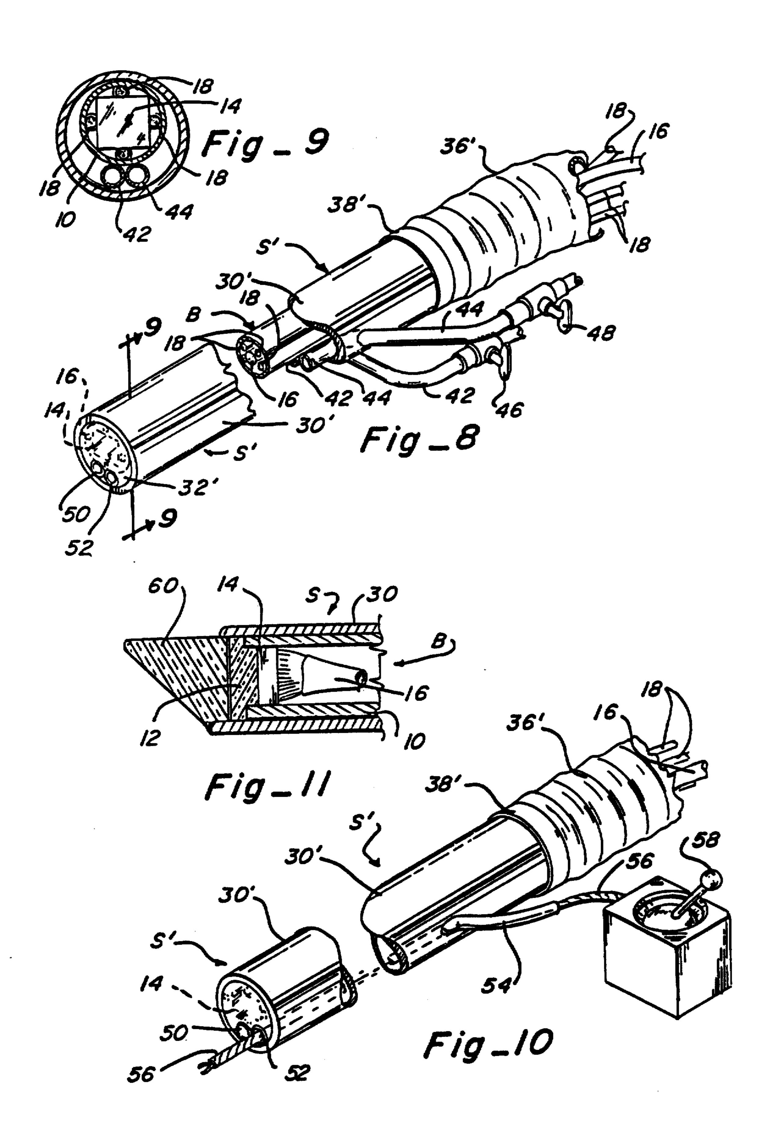
Sidall et al. U.S. Pat. No. 4,741,326 discloses a further flexible sheath which is rolled up along the endoscope and does not provide sterility or protection of the entire endoscopic device.
