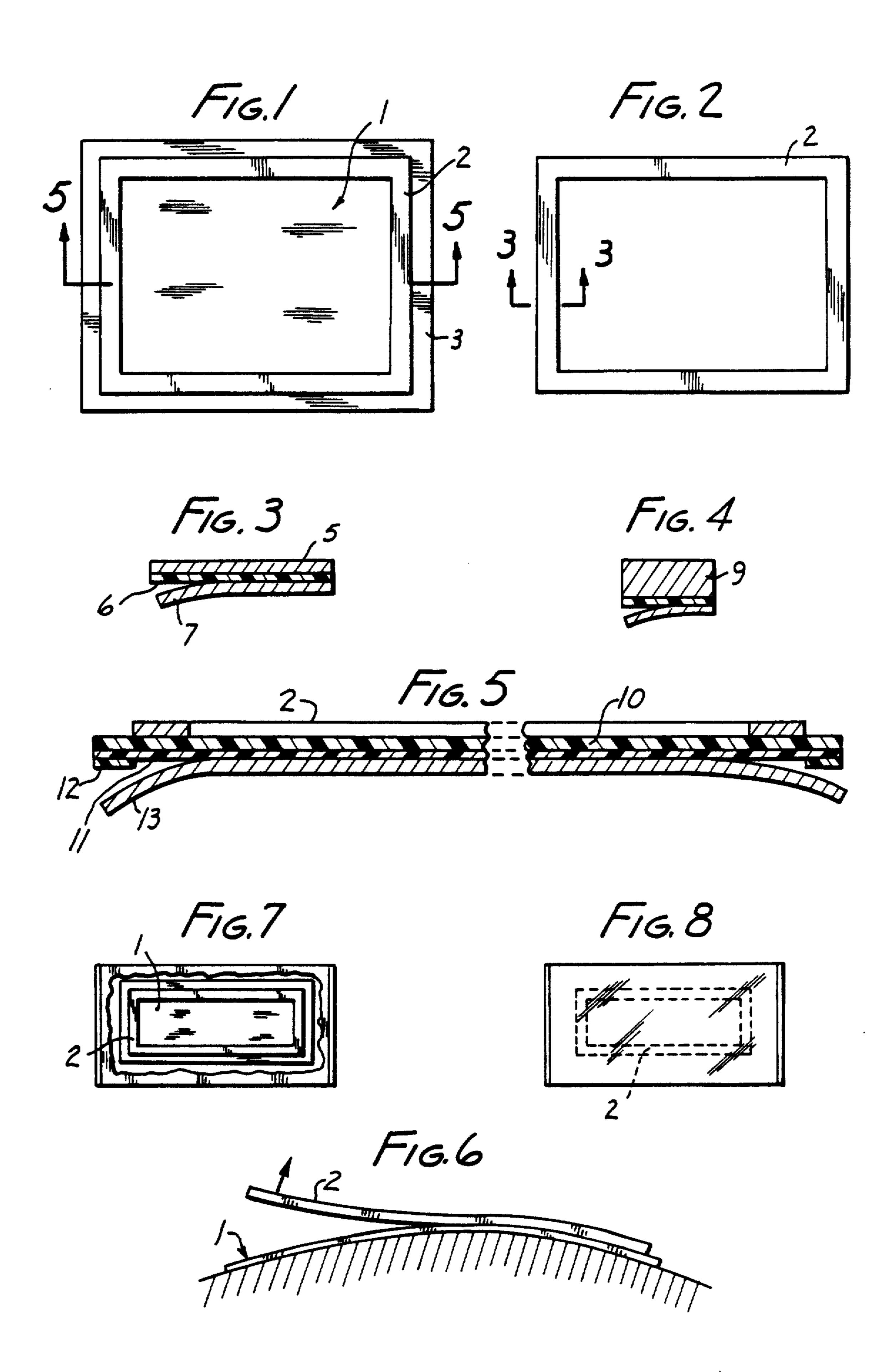
frame back 9 is of a relatively thicker material, but not as wide as the FIG. 3 embodiment.
