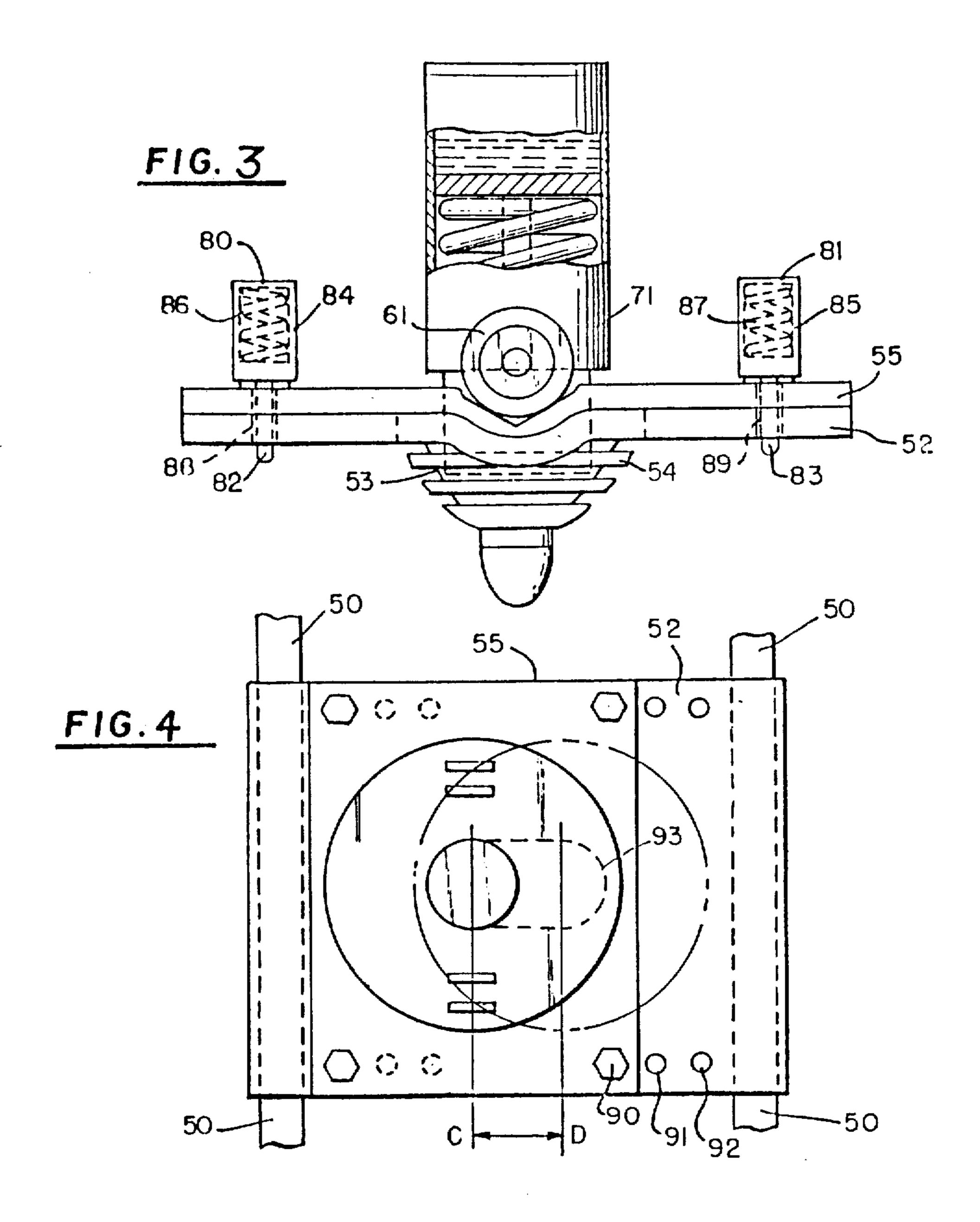
64 which are mounted to the cross-bar by means of sleeves 65 and 66. The cross member 62 rotates about pivot pin 58 as the trailer varies its yaw angle.
