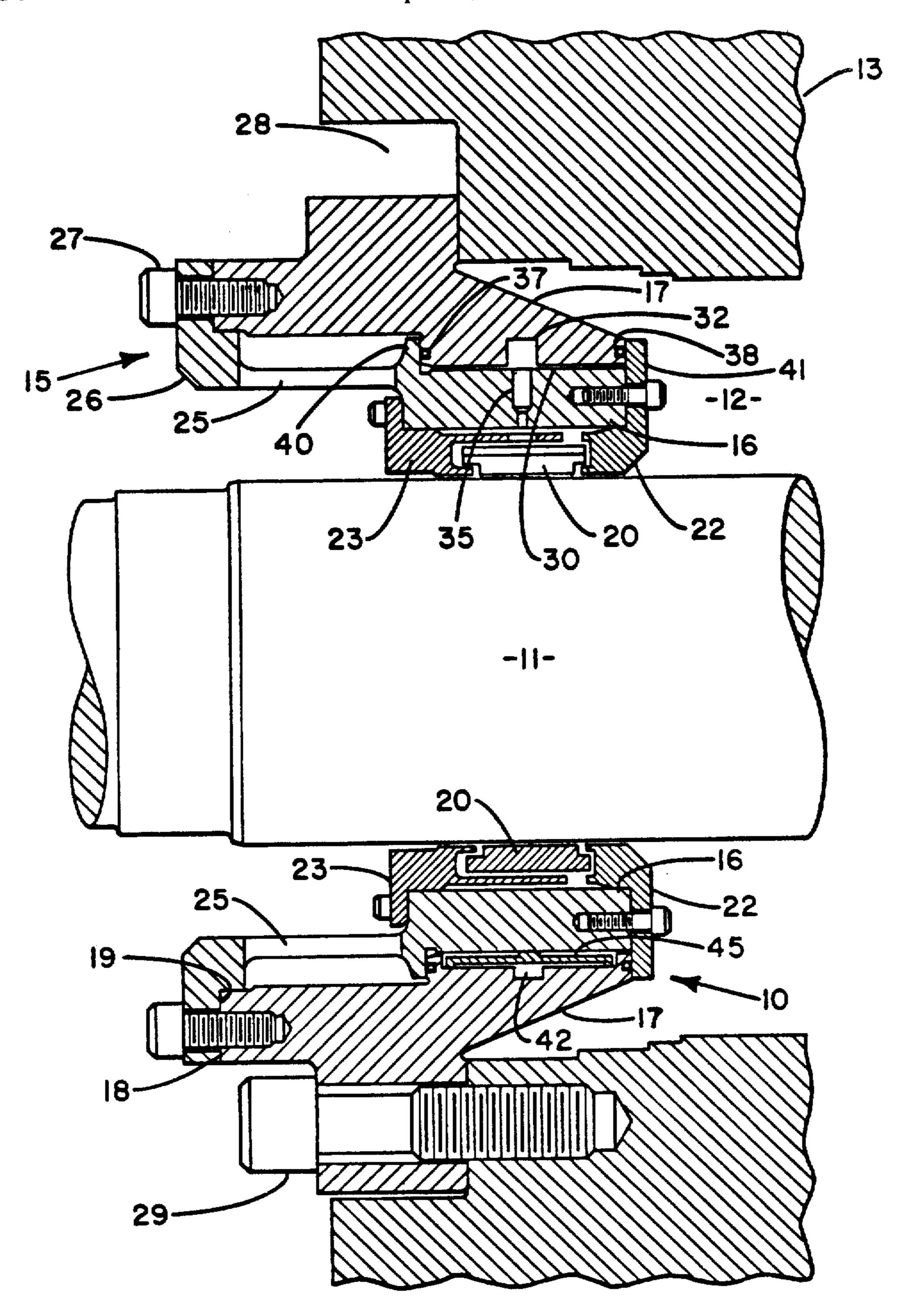
trating a flexible damped bearing assembly encompassing the teachings of the present invention.
