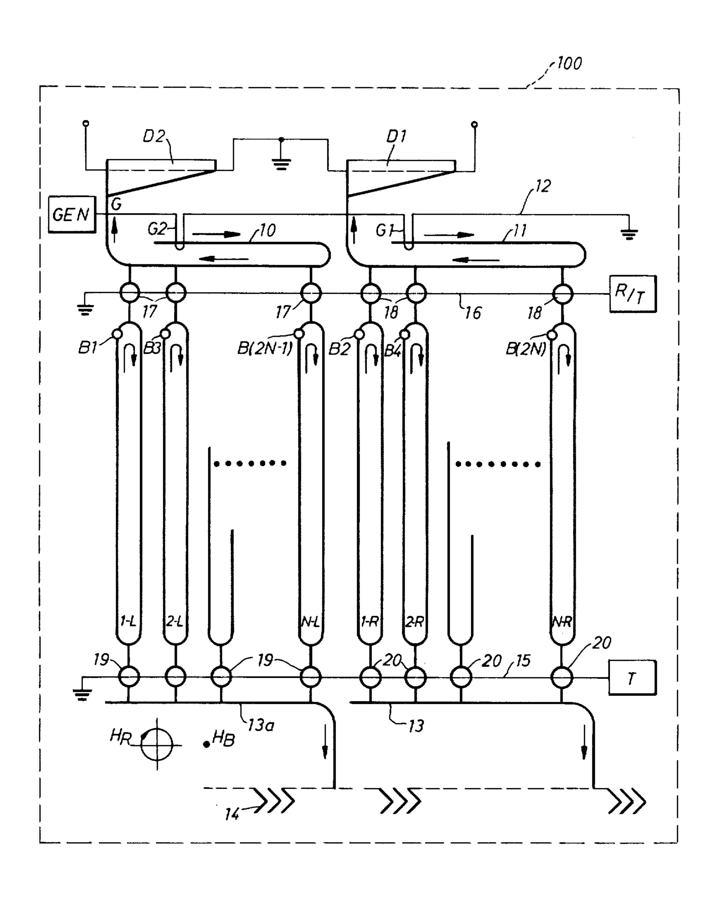
tion in the other access loop is transferred into the associated storage loops at a different time. I alternate bubbles are stored in opposite halves of the device.
