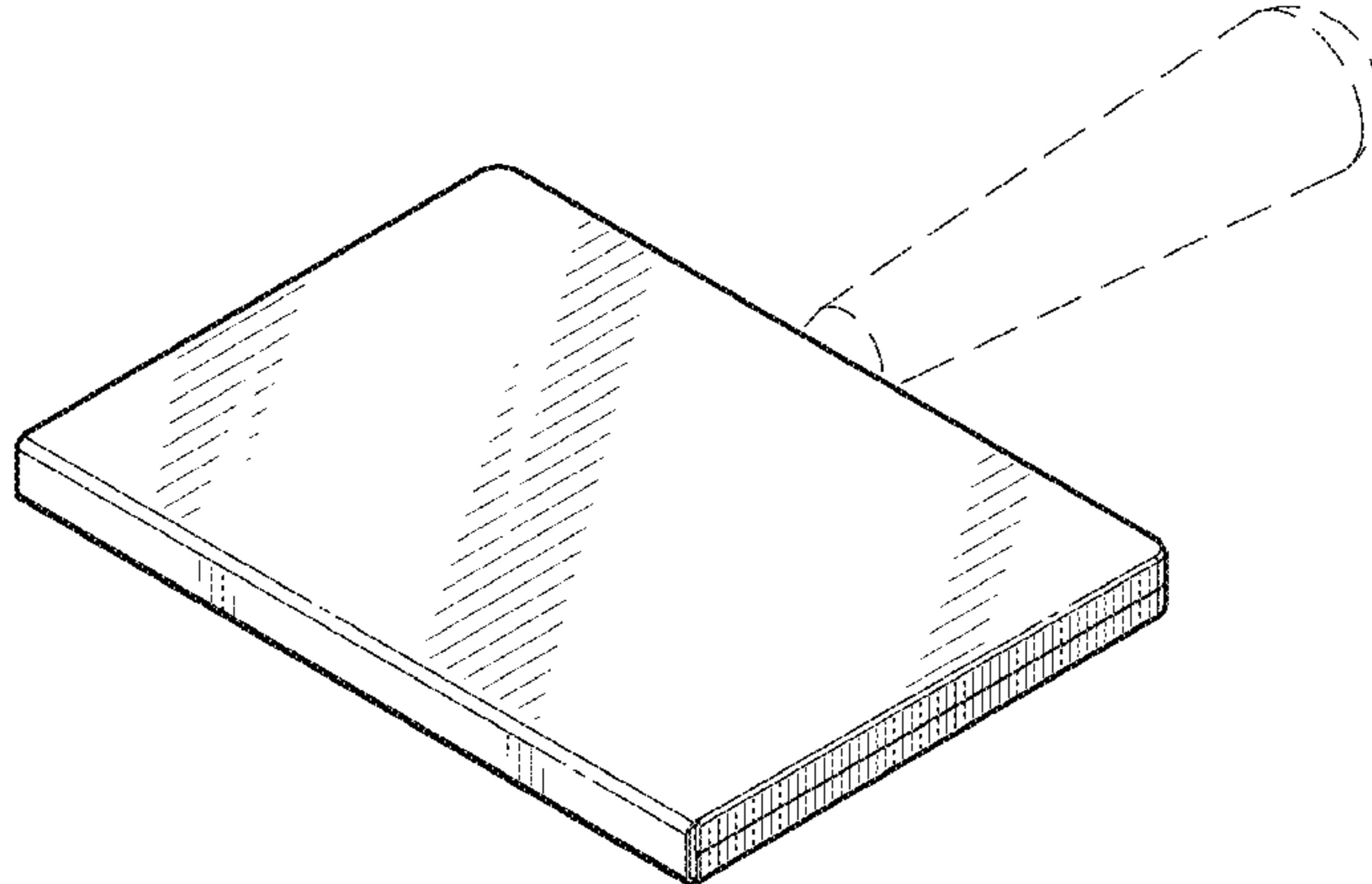
The claimed drywall knife case is used to protect and cover a drywall knife, which is also referred to as a putty knife, a taping knife, or a joint knife.
