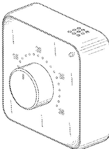
FIG. 18 is a second side view of the temperature controller of FIG. 15;
