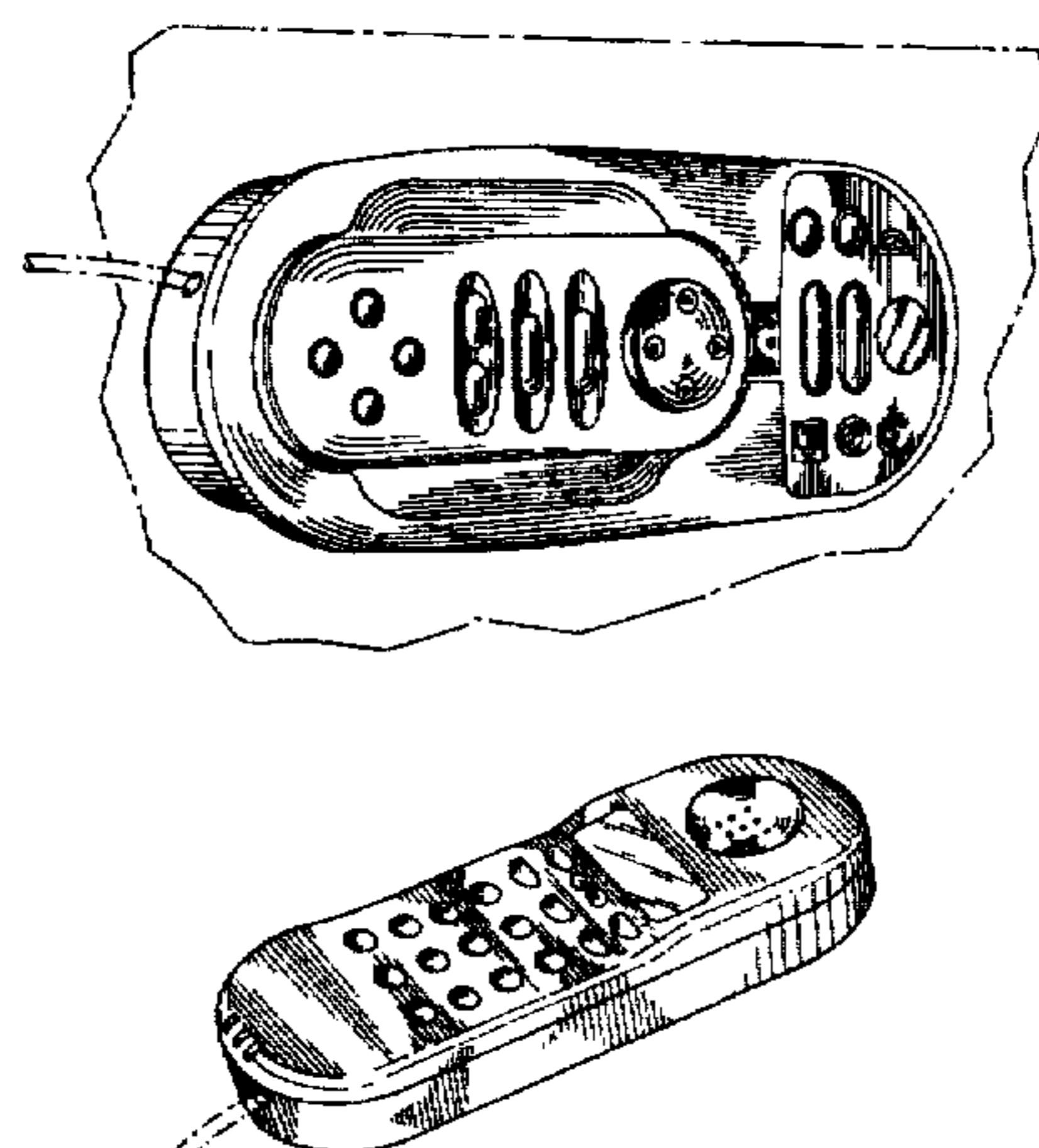
FIG. 8 is an exploded view of the interactive display controller and telephone handset unit of FIG. 1, featuring the top, left and front perspective views of the passenger control handset upon removal from the handset compartment; and, FIG. 9 is top, right and rear perspective views of the passenger control handset in FIG. 8;
