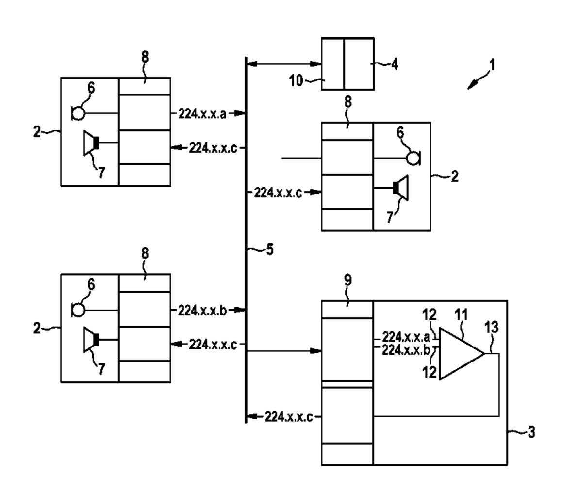
an output channel (13), whereby each input channel (12) can be assigned to a audio stream from one active audio device (2) and whereby the mixing unit (11) is operable to mix the audio streams from the plurality of input channels (12) into a common audio stream and to output the common audio stream to the output channel (13), whereby the audio streams from the active audio devices (2) to the processing device are transmitted by a multicast transmission.
