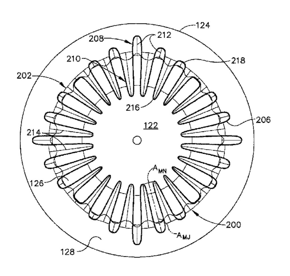
immersion lobe. The first bypass immersion lobe has a first crown contour line extending from the forward end to the aft end of the mixer, and the second bypass immersion lobe has a second crown contour line extending from the forward end to the aft end of the mixer. The first crown contour line is different than the second crown contour line.
