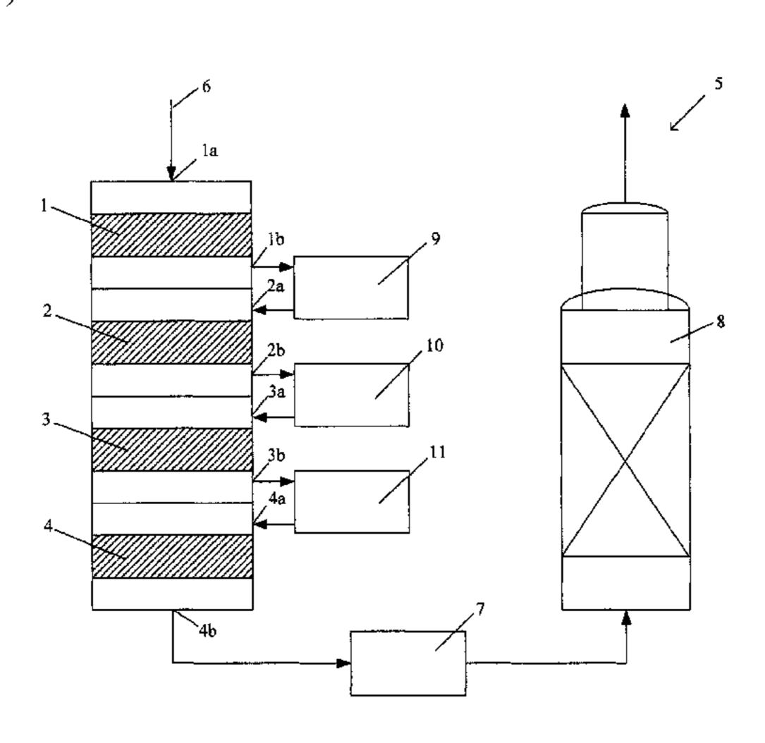
vanadium oxide catalyst and the last catalyst bed or beds comprise platinum catalyst operating at a much lower temperature than the initial beds.
