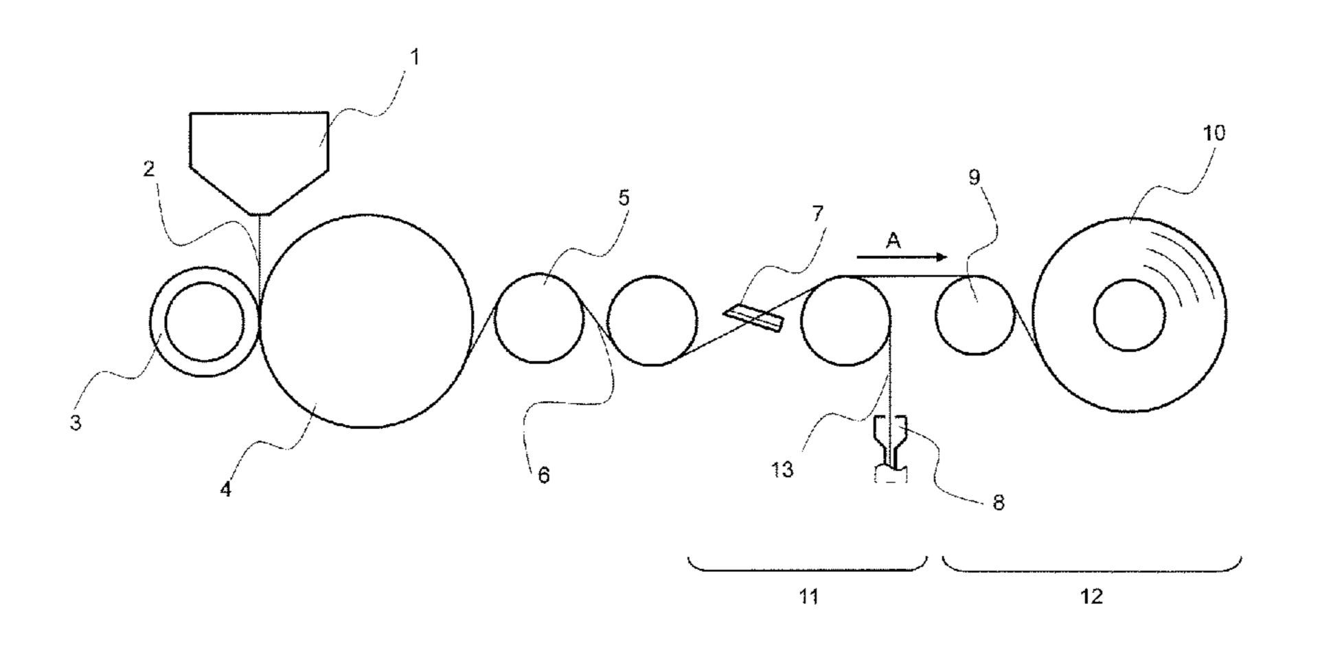
surface of a nip roller (3) to 2-8 µm and the mean distance (Sm) between protrusions and depressions thereof to no more than 90 μm.
