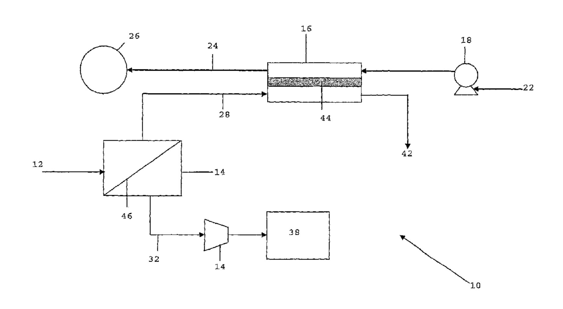
absorption unit to produce a hydrocarbon-rich gas phase and a liquid absorbent phase containing said carbon dioxide. The present disclosure also relates to a system for doing the same.
