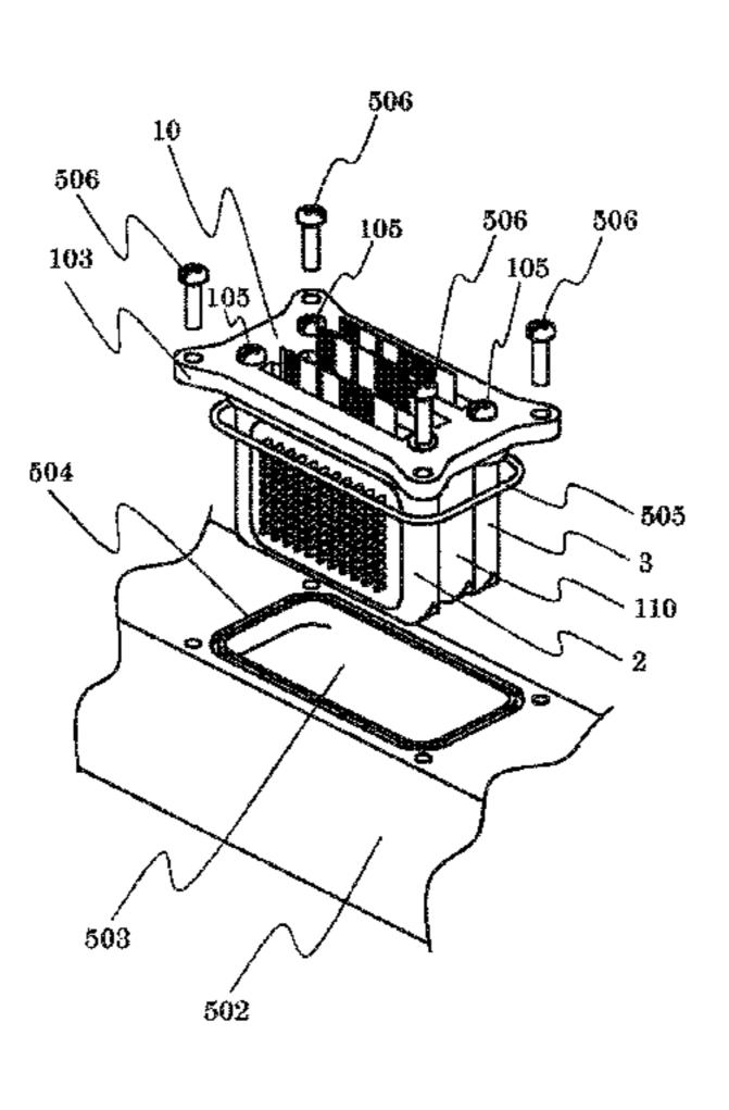
case is connected to the first flange portion so as to provide a first flow path space for allowing a coolant to flow between the second case and the first case, and the first flange portion is fixed to the fixing member while supporting the first case and the second power semiconductor module.
