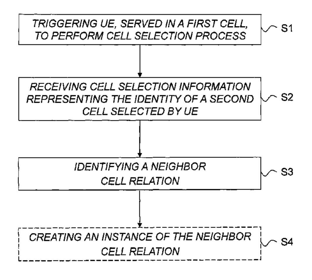
way, an efficient way of detecting a neighbor cell relation between different radio access technologies is provided.
