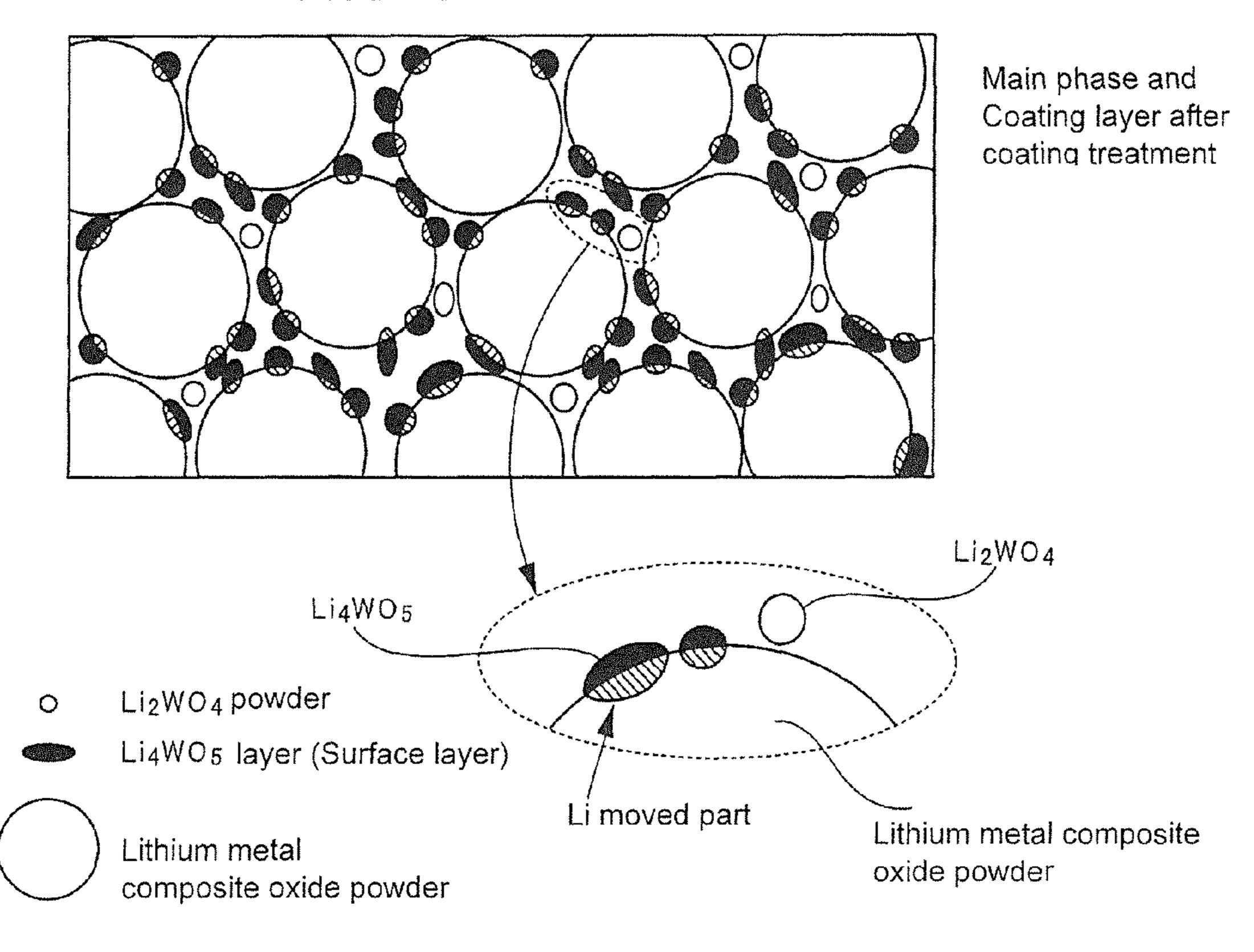
POSITIVE-ELECTRODE MATERIAL FOR NONAQUEOUS-ELECTROLYTE SECONDARY BATTERY, METHOD FOR MANUFACTURING THE SAME, AND NONAQUEOUS-ELECTROLYTE SECONDARY BATTERY USING SAID POSITIVE-ELECTRODE MATERIAL
