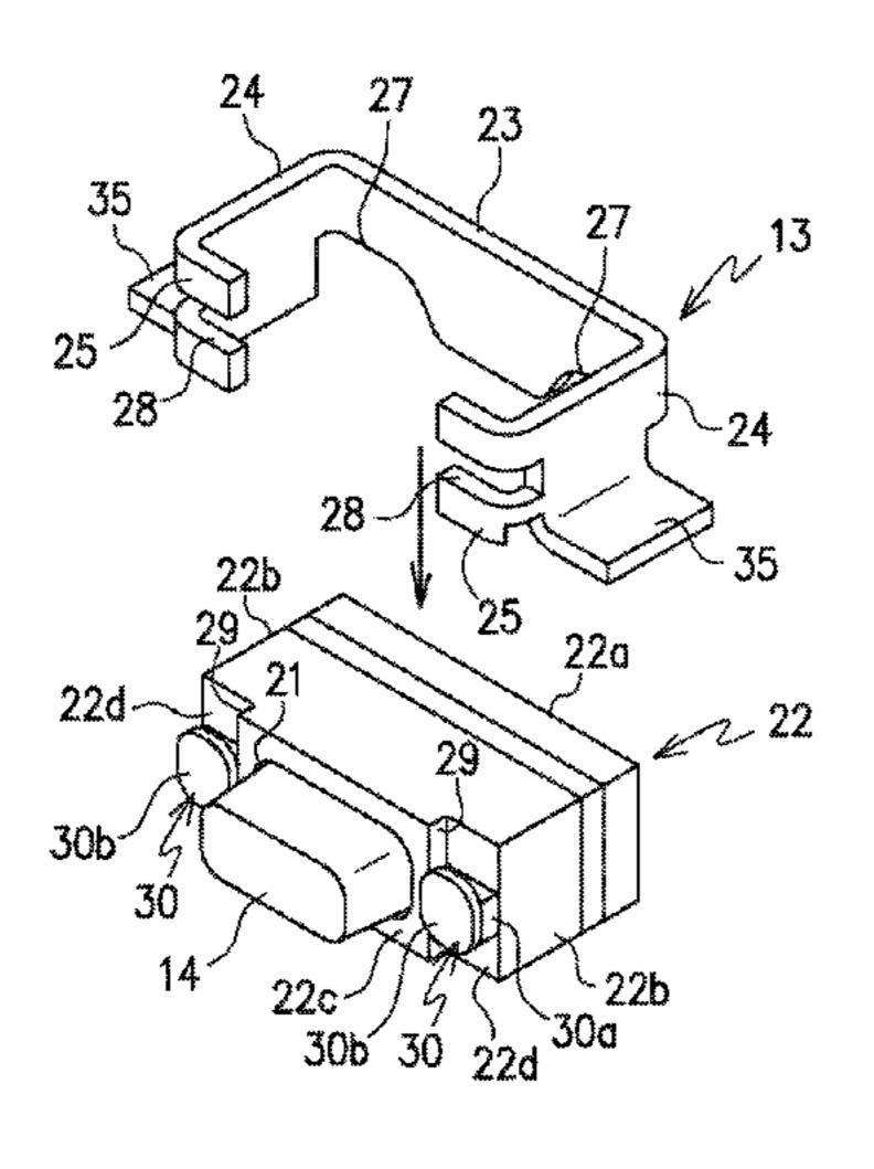
the housing. Both ends of the holding frame are secured to front-surface side portions of the housing on both sides of the push-button member.
