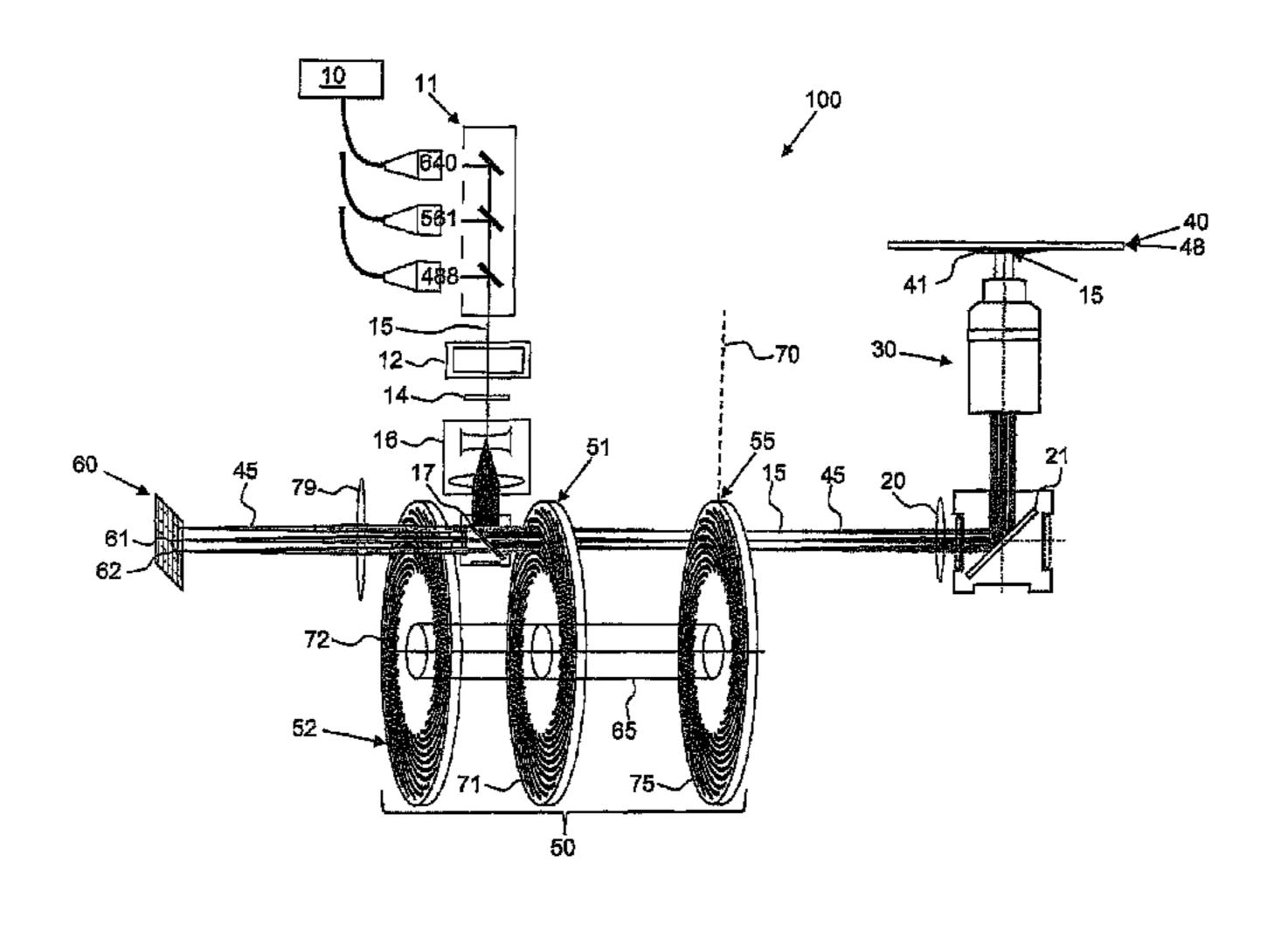
opposite to one another. Sample regions spaced apart from one another can be examined simultaneously, such that both a beam path of the sample light from the sample plane to the detector device and a beam path of the illumination light from the light source to the sample plane run via the first optical arrangement and only one of these two beam paths runs via the second optical arrangement.
