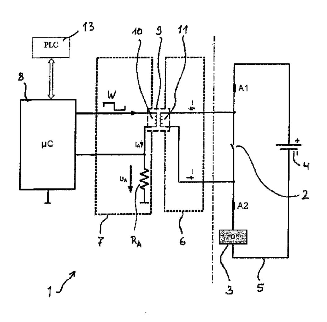
measured value  $(U_A)$  proportional to the current  $(I_A)$  flowing through the primary winding (10).
