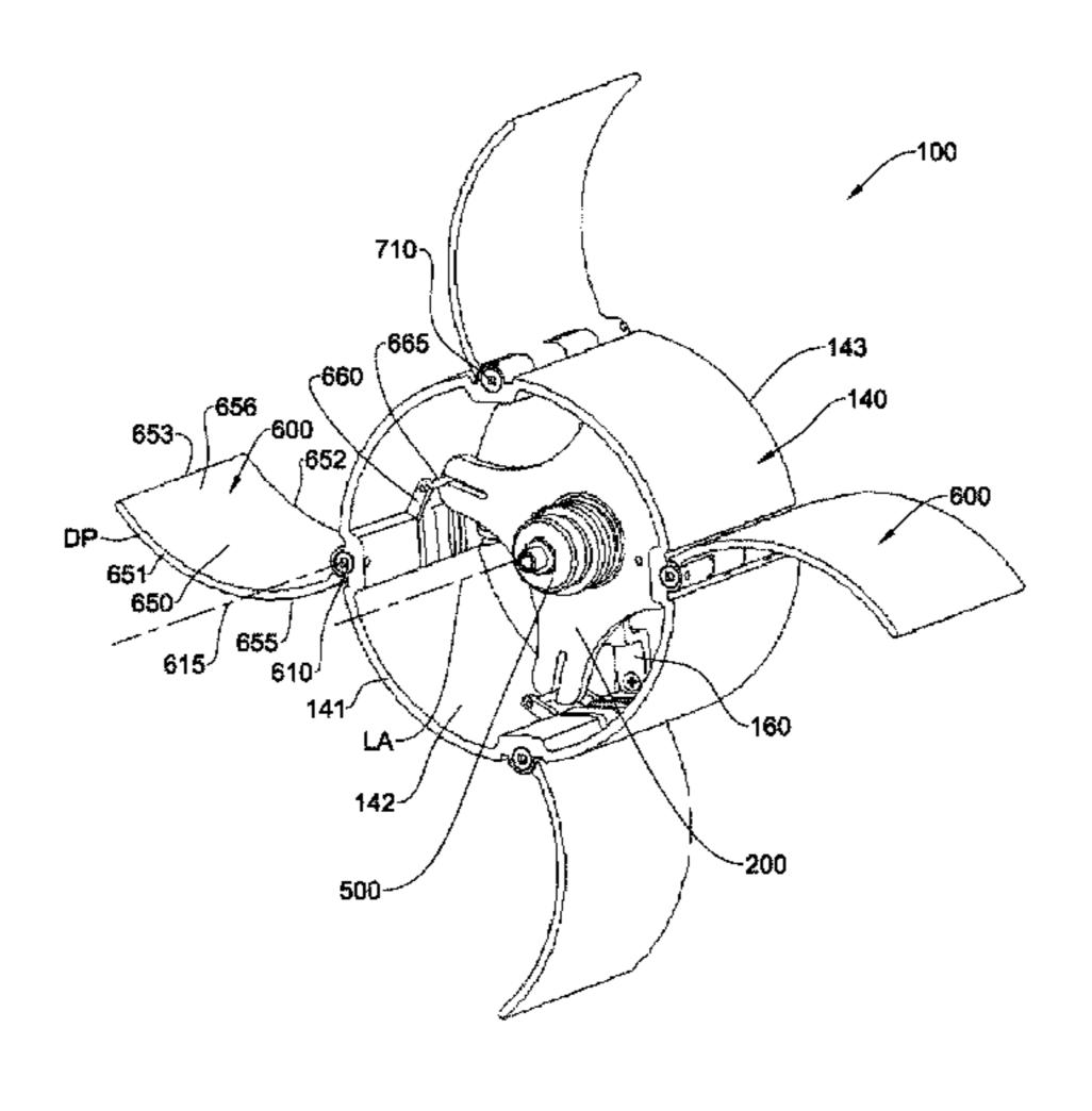
position, and the pivoting of each fin from the respective the stowed position to the respective the deployed position, are concurrent. The second mechanical stop arrangement is for locking the fin assemblies in the respective deployed positions responsive to the actuator plate pivoting from the first pivot position to the second pivot position.
