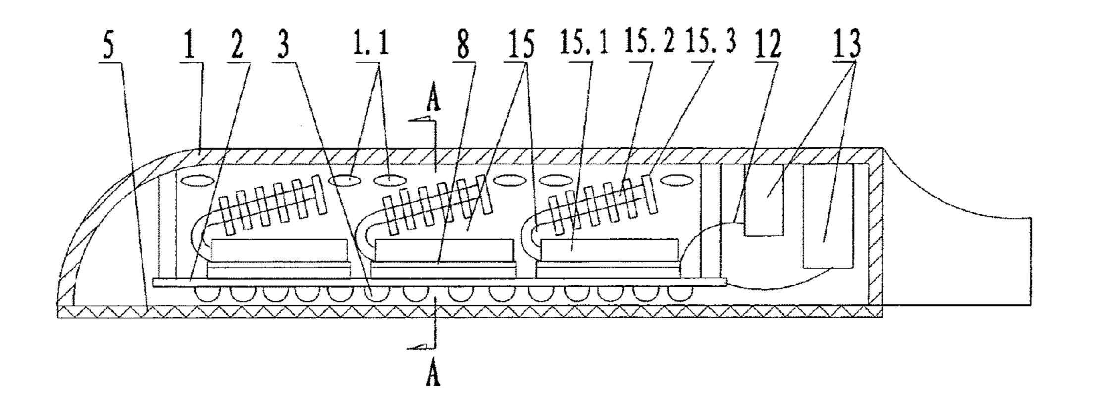
P-type semiconductor element (7), then lower beryllium-oxide ceramic wafer (9) is attached, through graphene thermal conductive greaseon layer (4), on backside of circuit board (2) which is mounted with LED bulbs (3), and heat sink (15) is mounted on upper beryllium-oxide ceramic wafer (8), then circuit board (2) together with heat sink (15) are mounted into street lamp housing (1).
