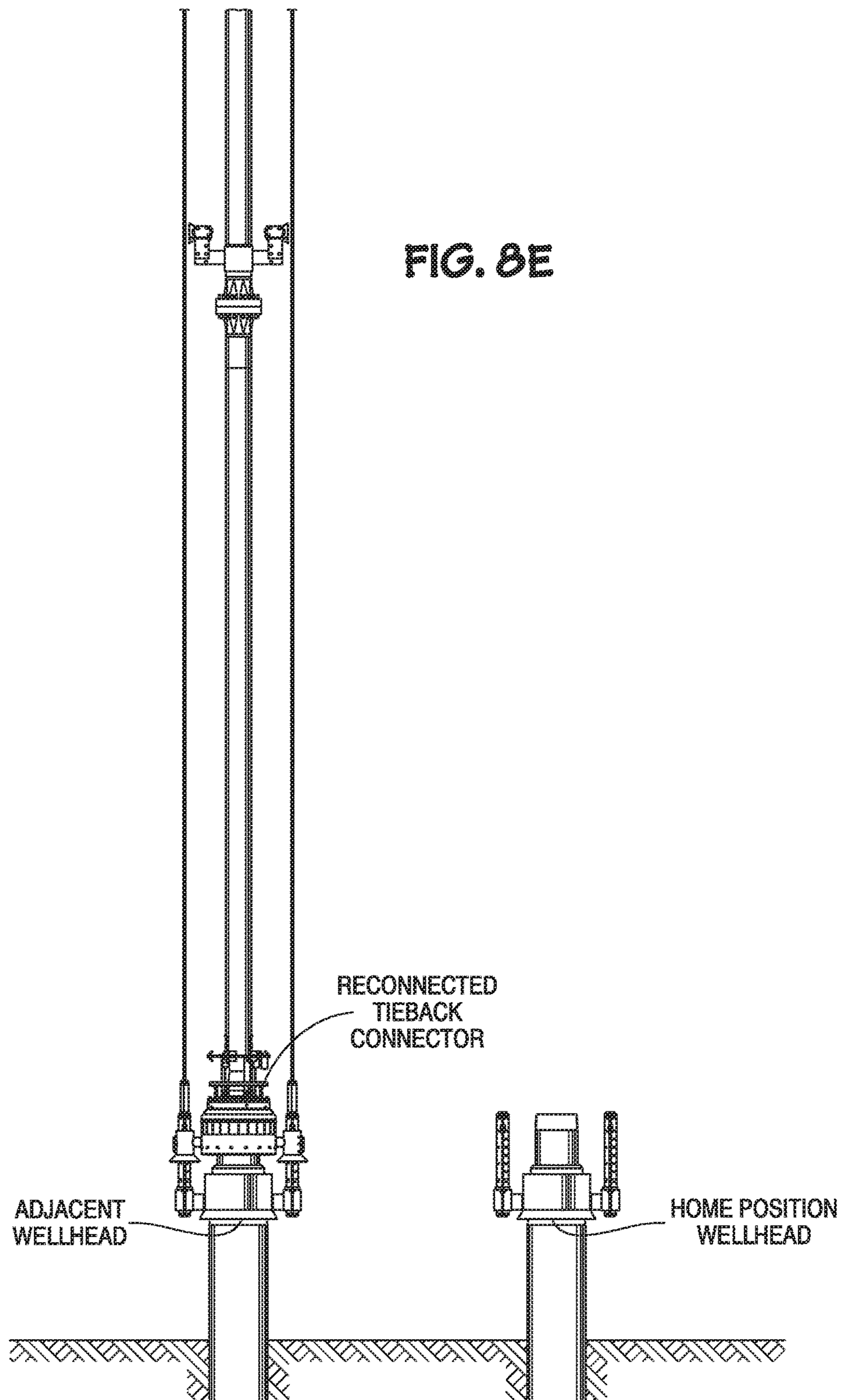
STEP 5: TIEBACK CONNECTOR LOWERED ONTO WELLHEAD GUIDED BY WIRE ROPES.
