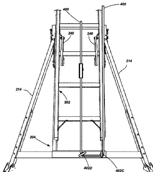
front of the rungs. A fall arrest mechanism, or an ascender device, may be coupled with the section of rope extending up the ladder between the rails and in front of the rungs.
