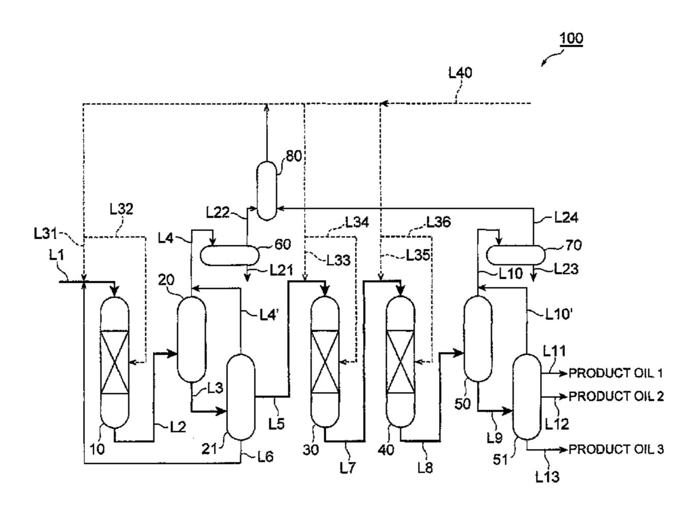
step of fractionating the hydrocracked oil into a base oil fraction comprising the hydrocracked product and a heavy fraction comprising the heavy matter and being heavier than the base oil fraction, respectively, a third step of isomerization dewaxing the base oil fraction from the fractionation in the second step to obtain a dewaxed oil, wherein the heavy fraction from the fractionation in the second step is returned to the first step as a part of the stock oil.
