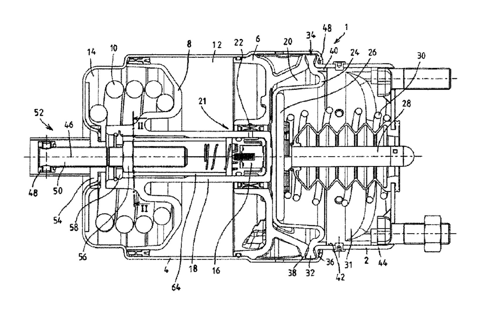
bushing and between an outer polygonal profiled section of the outer circumference of the intermediate bushing in the circumferential direction and a complementary circumferential inner polygonal profiled section on the inner circumference of the spring brake piston tube.
