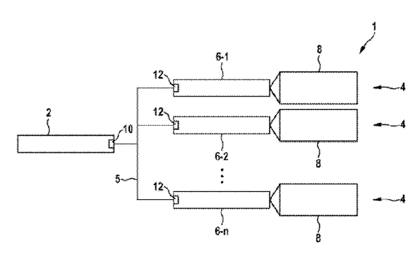
6-2, ..., 6-n) using the differential values and the reference measurement value. A computer program, a battery management system (1) and a battery which are designed to carry out the method are also described.
