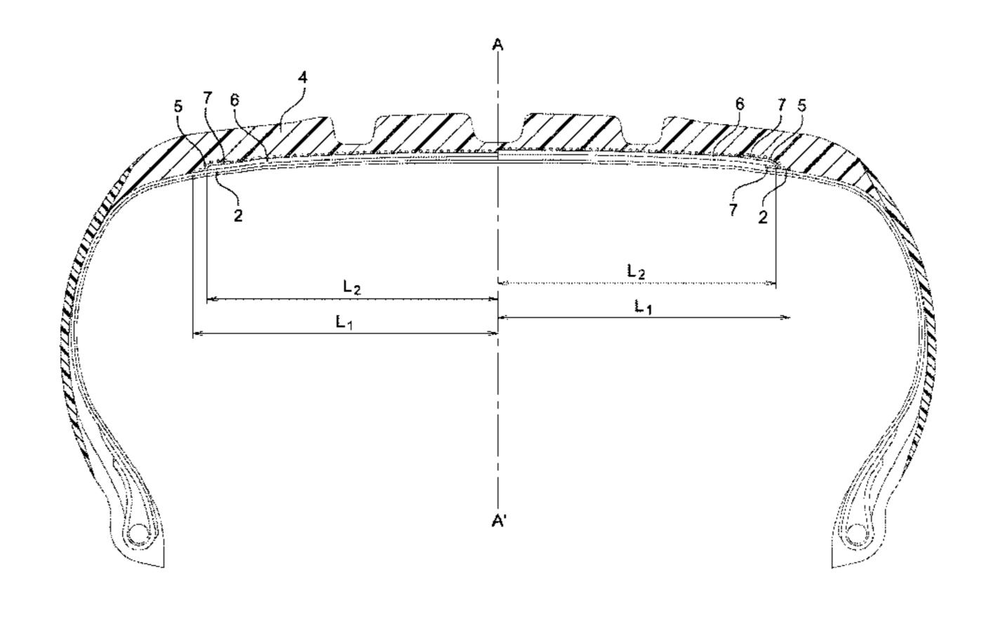
reinforcing elements, parallel two by two, forming an angle at most equal to 7° with respect to the circumferential direction,
