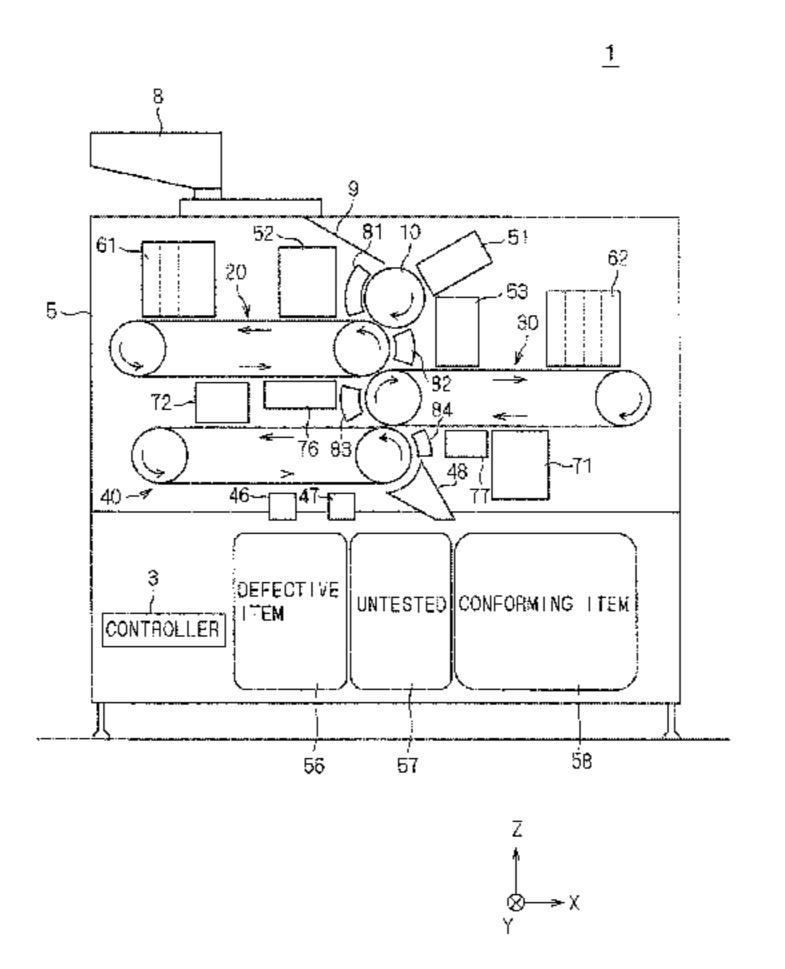
head performs back-side printing process on a back side of a tablet to conform to a direction on the back side same as the predetermined direction.
