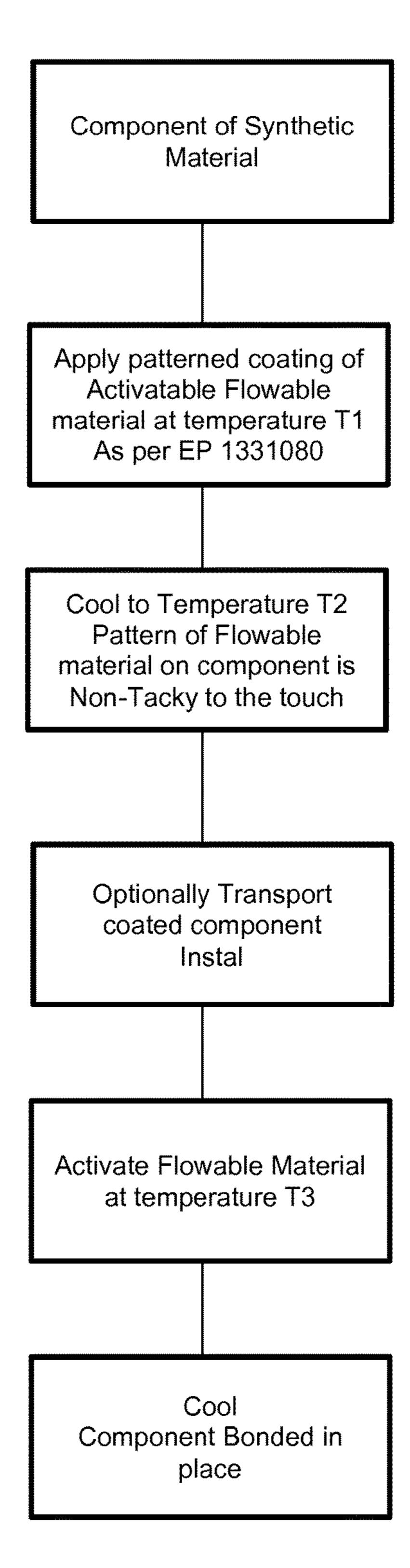
The material from which the component is made must withstand temperatures T1, T2 and T3. T3 must be greater than T1.
