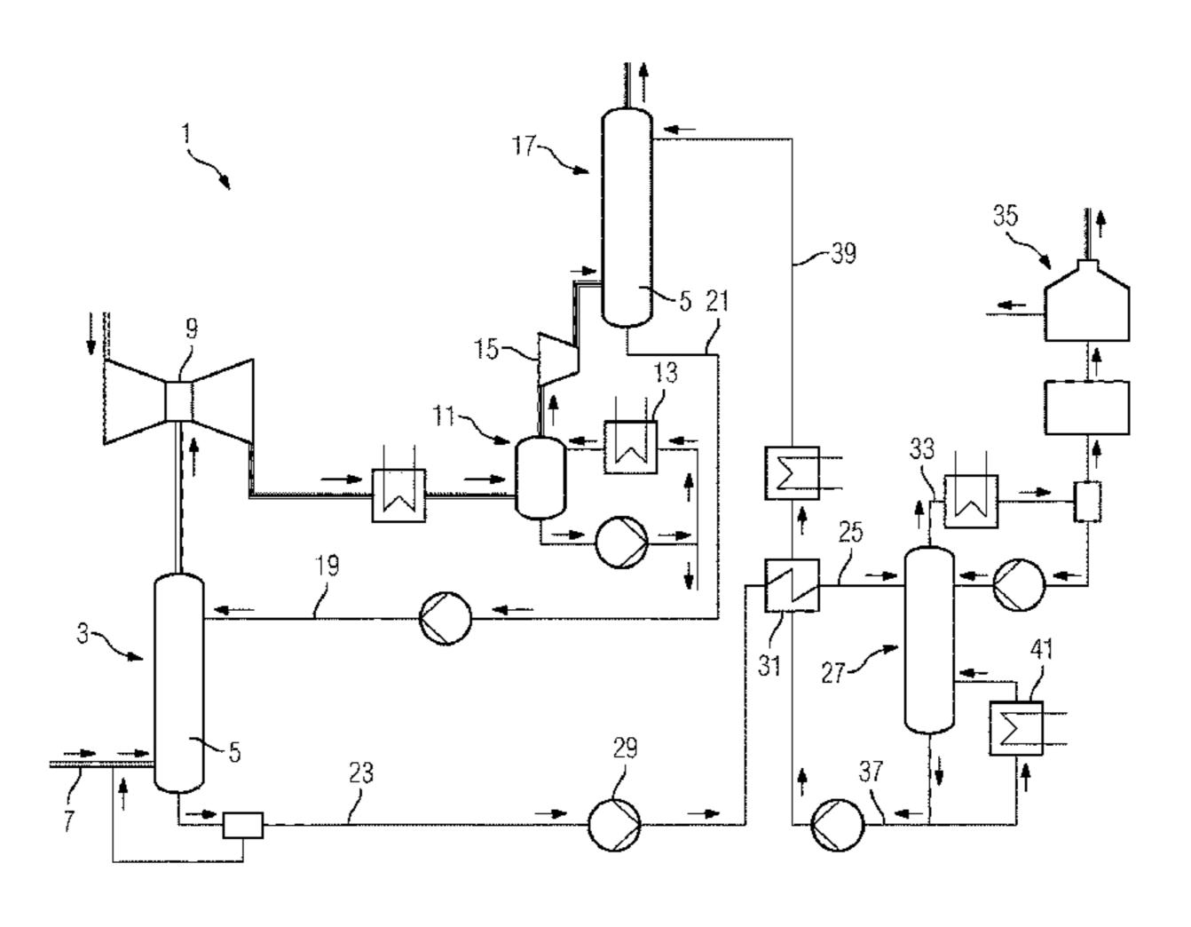
has a first absorber and a second absorber flow-connected to one another for the exchange of absorption medium.
