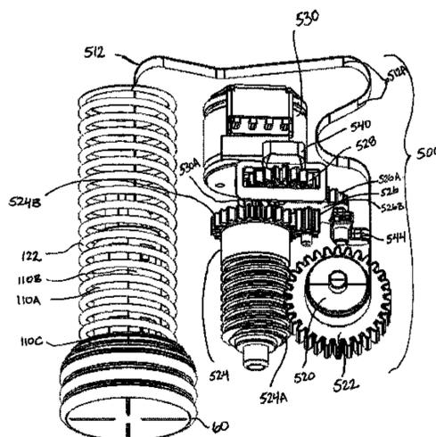
having a motor configured to drive the gear assembly to release the tether from the winch drum. The metering of the tether by the motor controls the rate or profile of drug delivery to a user. A drug delivery pump includes such a controlled delivery drive mechanism. A control system may be utilized to control the desired drug delivery rate/profile.
