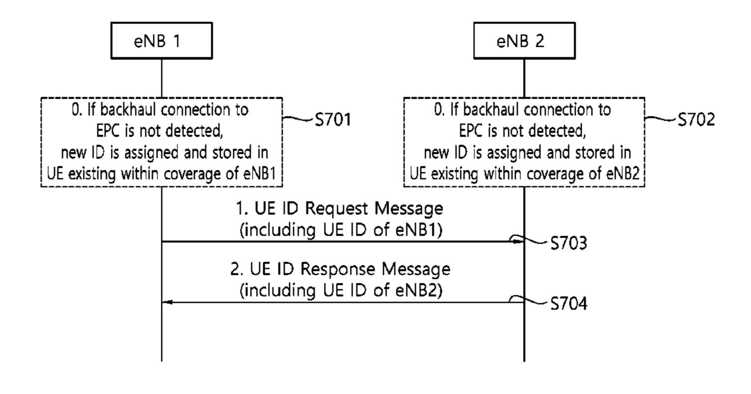
when a backhaul connection is not detected, the GUTI of the terminal in the service area of the first base station is transmitted to the second base station.
