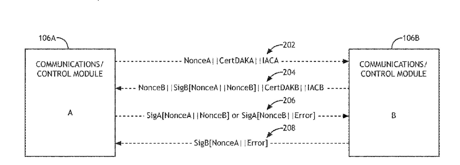
with the first and second nonces, a second device authentication key certificate, and a second identity attribute certificate; and transmitting an authentication datagram from the first communications/control module to the second communications/control module when the response datagram is valid, the authentication datagram including a second signature associated with the first and second nonces.
