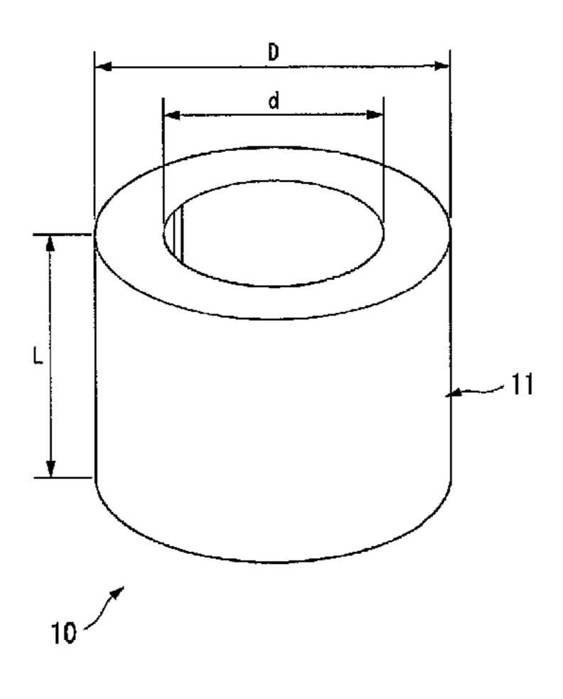
the cylindrical ingot, to form the cylindrical sputtering target material in which an average crystal grain diameter of an outer peripheral surface is from 10  $\mu$ m to 150  $\mu$ m and a proportion of the area of crystal grains having a crystal grain diameter more than double the average crystal grain diameter is less than 25% of the entire crystal area.
