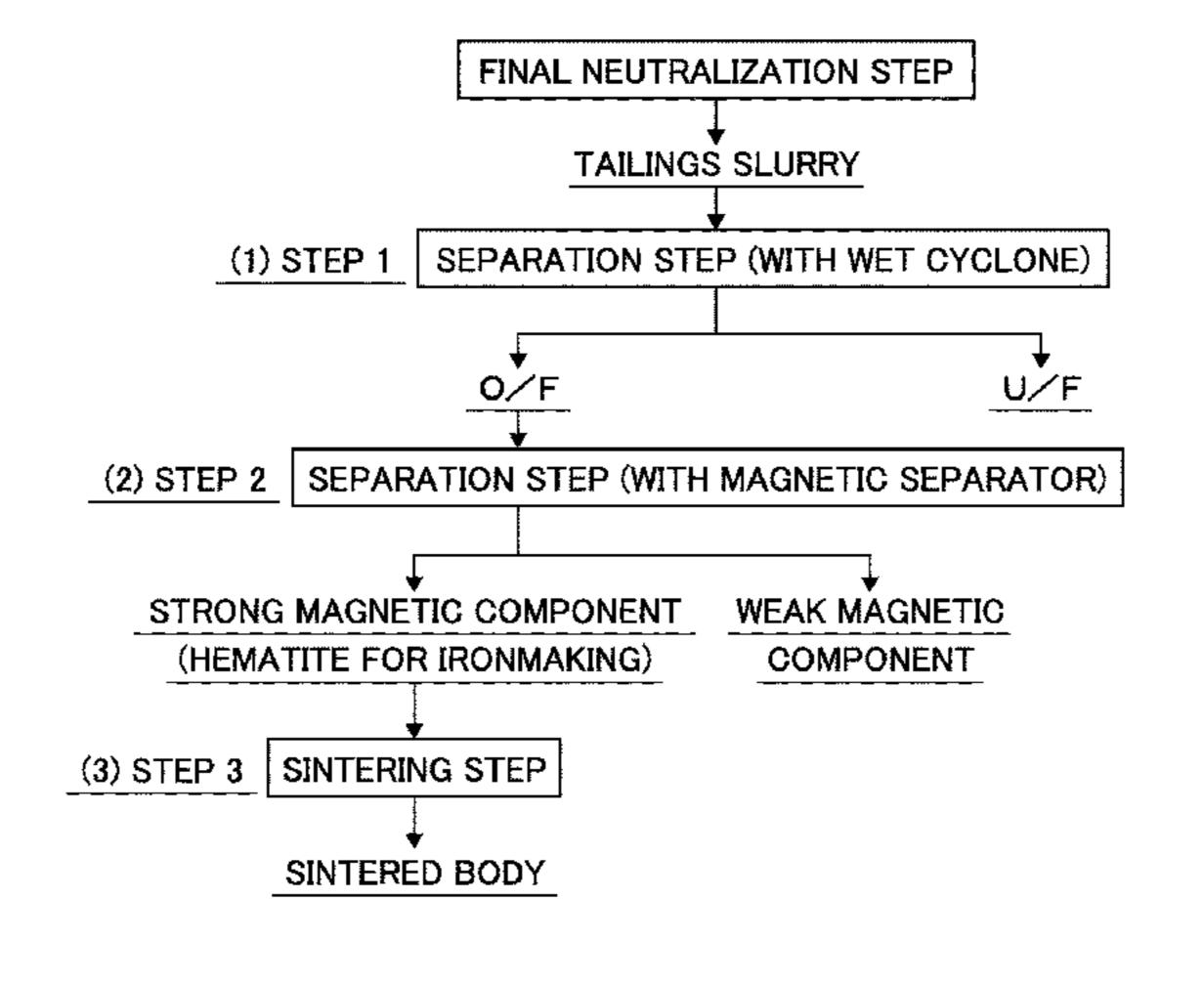
strong magnetic component and a weak magnetic component using a strong-magnetic-field magnetic separator utilizing magnetic force; and a third step of sintering the separated strong magnetic component at a temperature of 1150 to 1350° C. to form a sintered body.
