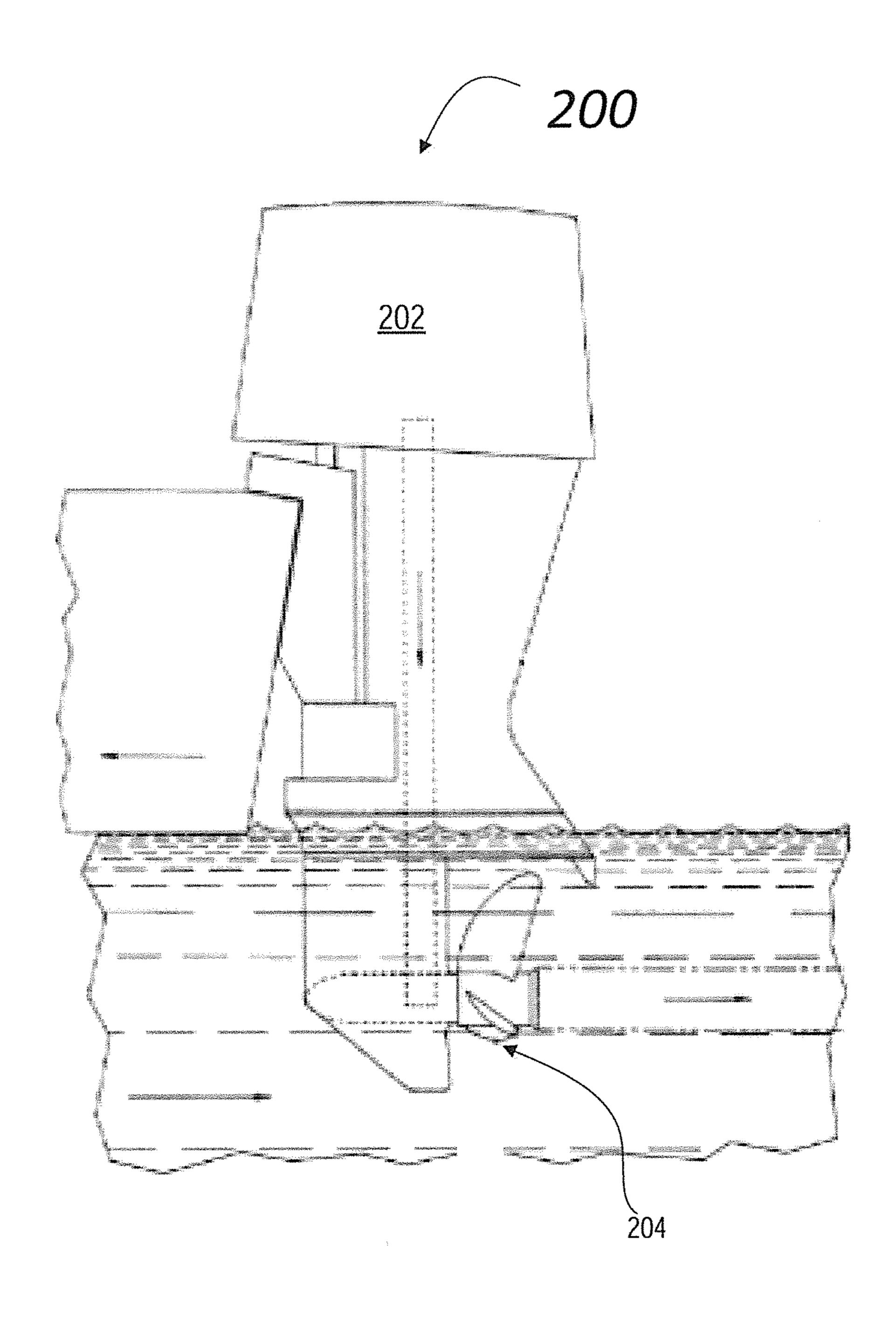
Fig. 2 (Conventional Through-the-Hub Motor with Propeller)
