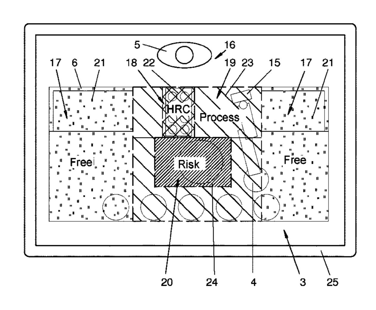
different zones (17, 18, 19, 20) having differently high levels of risk of hazard from the industrial robot (4) for the worker (5). The industrial robot (4) is suitable for human-robot cooperation.
